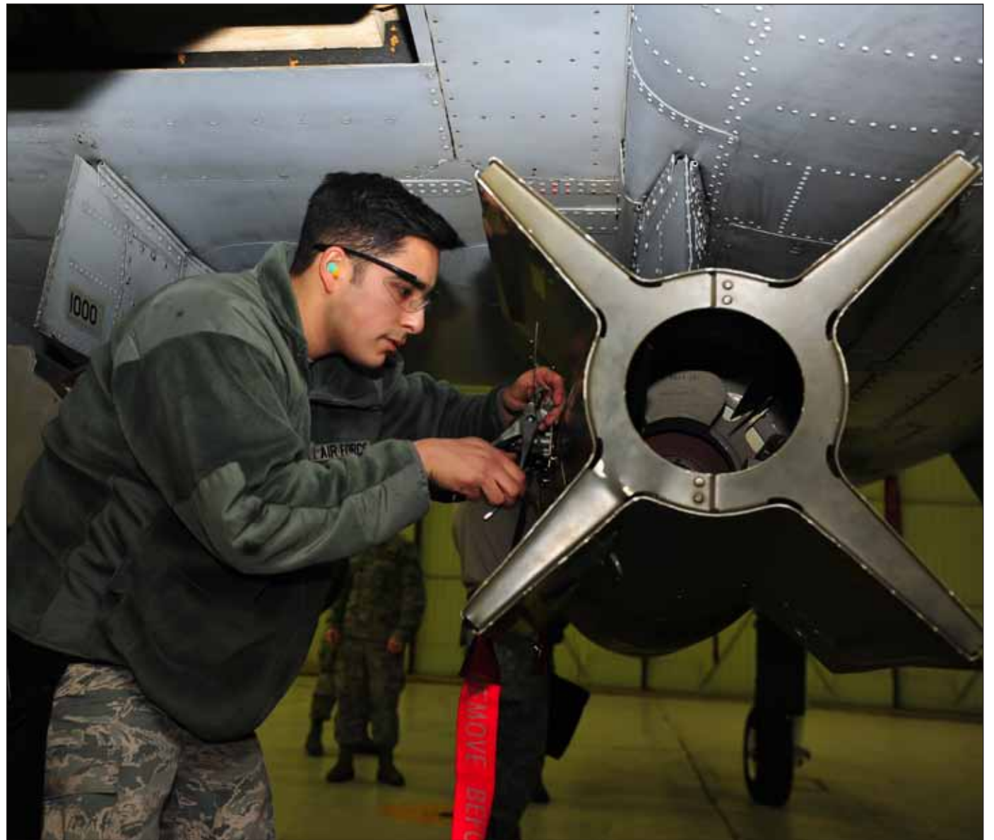
Senior Airman Dylan Logsdon, 51st Maintenance Operations Flight load crew member, cuts an arming wire to approximately one inch during the arming process during a weapons standardization inspection Dec. 16, 2014, at Osan Air Base, Republic of Korea. The load crew members are required to be recertified on the 15 different munitions every 30-days. (U.S. Air Force photos by Senior Airman David Owsianka)
