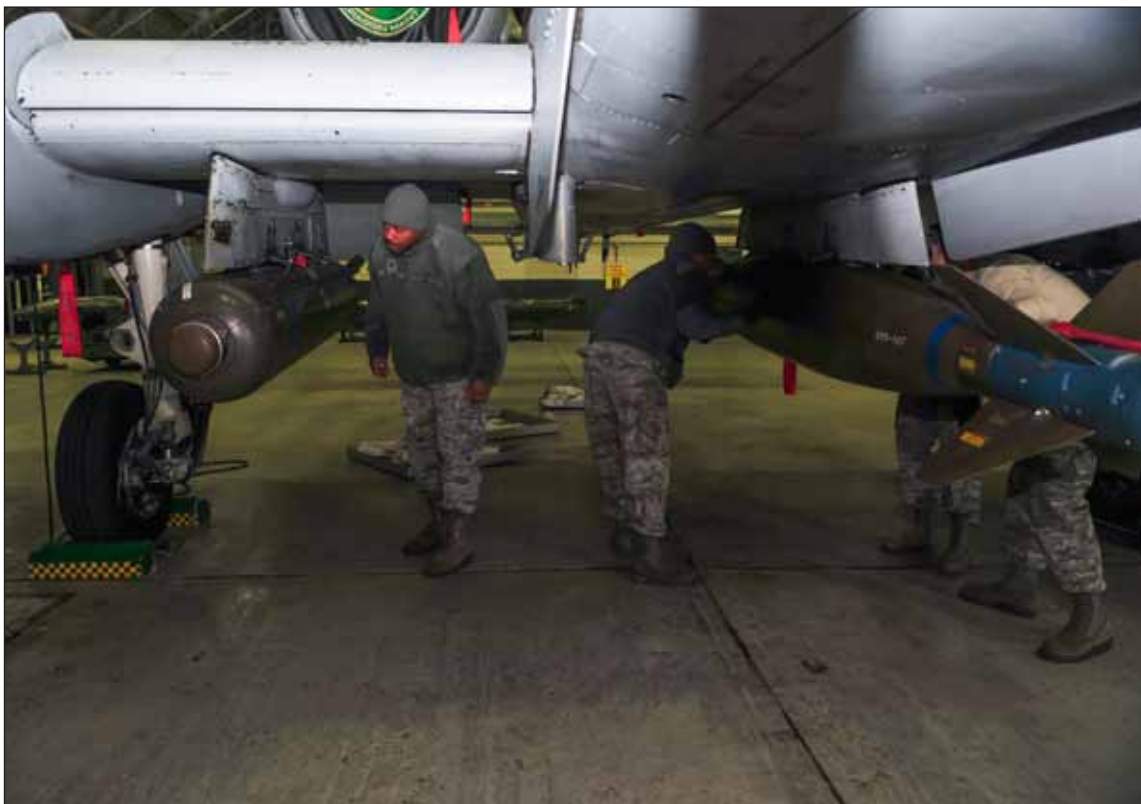
Weapons standardization members inspect the completed work of the 51st Maintenance Operations Flight load crew members Dec. 16, 2014, at Osan Air Base, Republic of Korea. The load crew members are required to be recertified on the 15 different munitions every 30-days.
