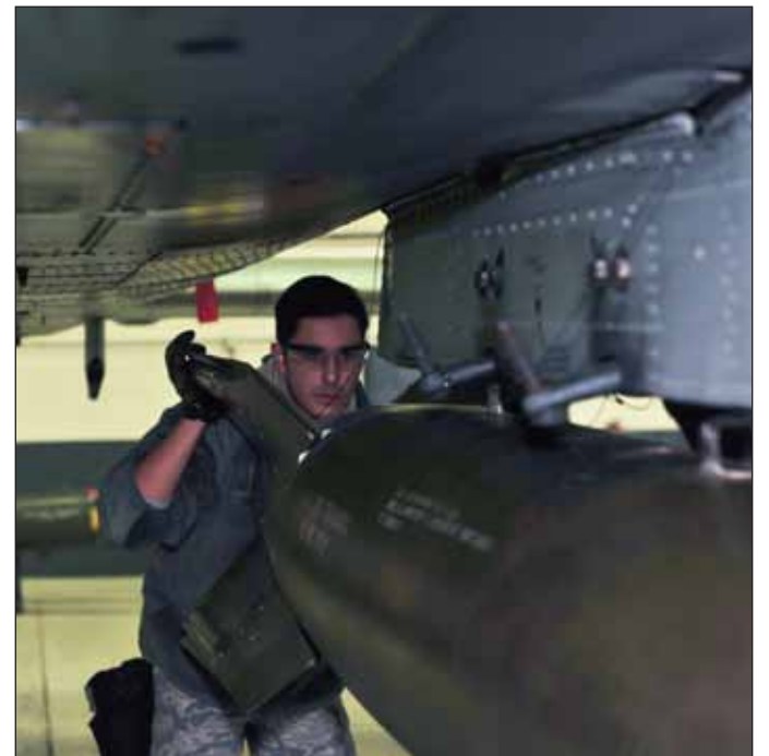
Senior Airman Dylan Logsdon, 51st Maintenance Operations Flight load crew member, ensures the bomb is lined up with the bomb rack during a weapons standardization inspection Dec. 16, 2014, at Osan Air Base, Republic of Korea. Some of the criteria the Airmen have to complete to pass the inspection are loading the munitions in a certain amount of time, maintaining proficiency, ensuring they have checked off the required steps and safely completed the job.
