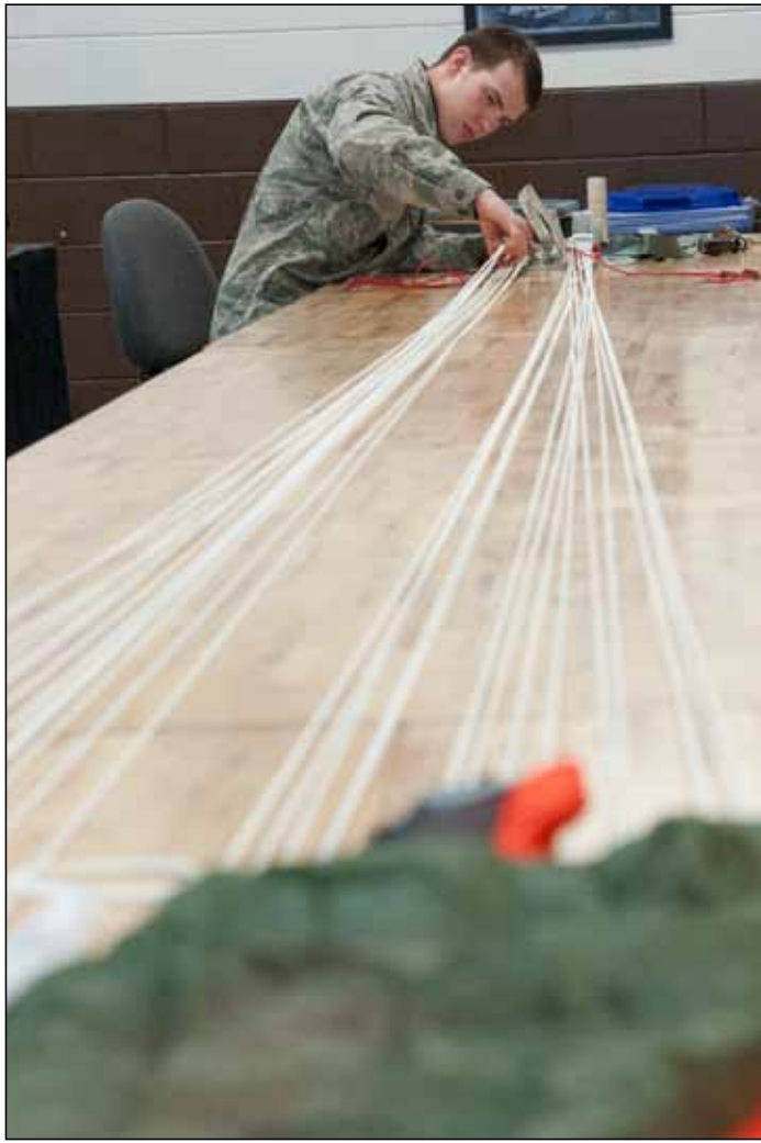
Senior Airman Mark Peterson, 51st Operations Support Squadron aircrew flight equipment journeyman, attaches a four line release lanyard onto a parachute at Osan Air Base, Republic of Korea, Jan. 20, 2015. The four line lanyards are used to help steer the parachute as well as release air from the canopy. (U.S. Air Force photo by Senior Airman Matthew Lancaster)
