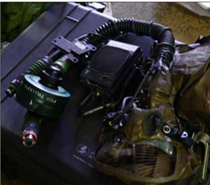
An Aircrew Eye and Respiratory Protection System sits on top of its container box May 4, 2015, at Osan Air Base, Republic of Korea. The AERP system provides aircrew with above the neck chemical and biological protection in the event of an attack during combat. The AERP system includes a hood, MBU12/P mask, C2 filter, an intercom for ground communication and a blower assembly that provides demisting.
