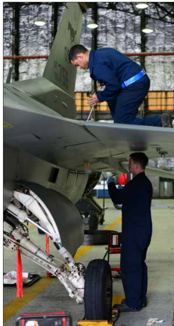
Above: Staff Sgt. Christian Rodriguez-Tanon, a Crew Chief assigned to the 51st Maintenance Squadron F-16 Phase Docks, directs a landing gear check at Osan Air Base, Republic of Korea, April 16, 2015. Crew chiefs work around the clock at depaneling and inspecting all standard carded items such as the wings, landing gear and fuselage as well as performing preventive maintenance on the jet as a whole. (U.S. Air Force photos by Staff Sgt. Amber Grimm)
