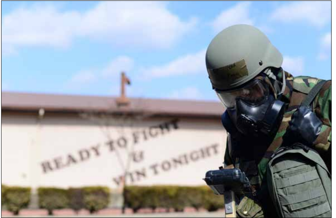
Above: Senior Airman Jonathan Caasi, 51st Civil Engineer Squadron emergency manager, checks M8 chemical detection paper during Operational Readiness Exercise Beverly Midnight 15-1 March 4, 2015, at Osan Air Base, Republic of Korea. M8 paper is used to identify if an area is contaminated with nerve and blister chemical agents. (U.S. Air Force photos by Senior Airman Matthew Lancaster)
