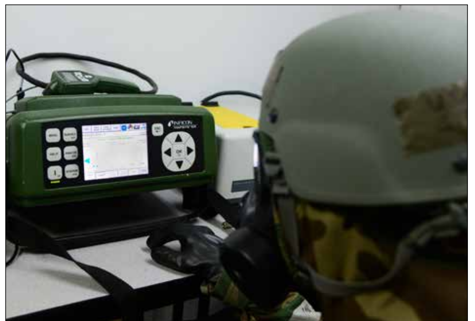
Staff Sgt. Steven Staab, 51st Aerospace Medicine Squadron NCO in charge of radiation, review the results the HAPSITE ER Chemical Identification System gave during Operational Readiness Exercise Beverly Midnight 15-1 March 4, 2015. The HAPSITE ER is used to test the air for any chemical contamination.
