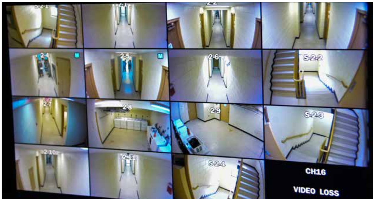
Closed circuit television imagery captured in dormitory building 1349 at Osan Air Base, Republic of Korea, April 22, 2015. With capabilities such as motion activation, low light capture, zoom, 1080 resolution and the ability to record up to a terabyte or roughly two weeks of data these CCTVs are an asset to ensuring the safety and wellbeing of residents. (U.S. Air Force photo by Staff Sgt. Jacob Barriero)
