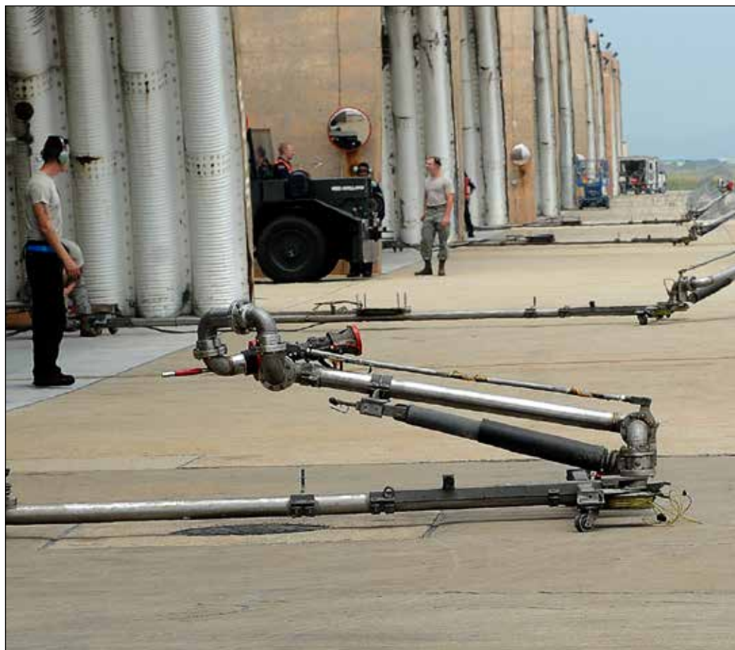
Above: Kunsan Airmen stand by to refuel F-16s during Surge Week at Kunsan Air Base, Republic of Korea, June 16, 2015. Pilots and maintainers conducted hot pit refueling to rapidly refuel each aircraft and allow it to complete a second sortie, thereby maximizing the sorties flown in a short amount of time.
