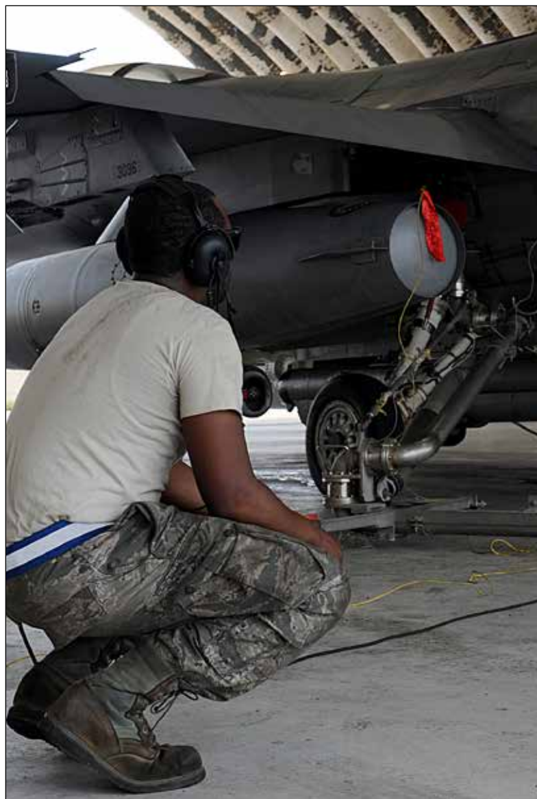
Above: Kunsan Airmen stand by to refuel F-16s during Surge Week at Kunsan Air Base, Republic of Korea, June 16, 2015. Pilots and maintainers conducted hot pit refueling to rapidly refuel each aircraft and allow it to complete a second sortie, thereby maximizing the sorties flown in a short amount of time.
