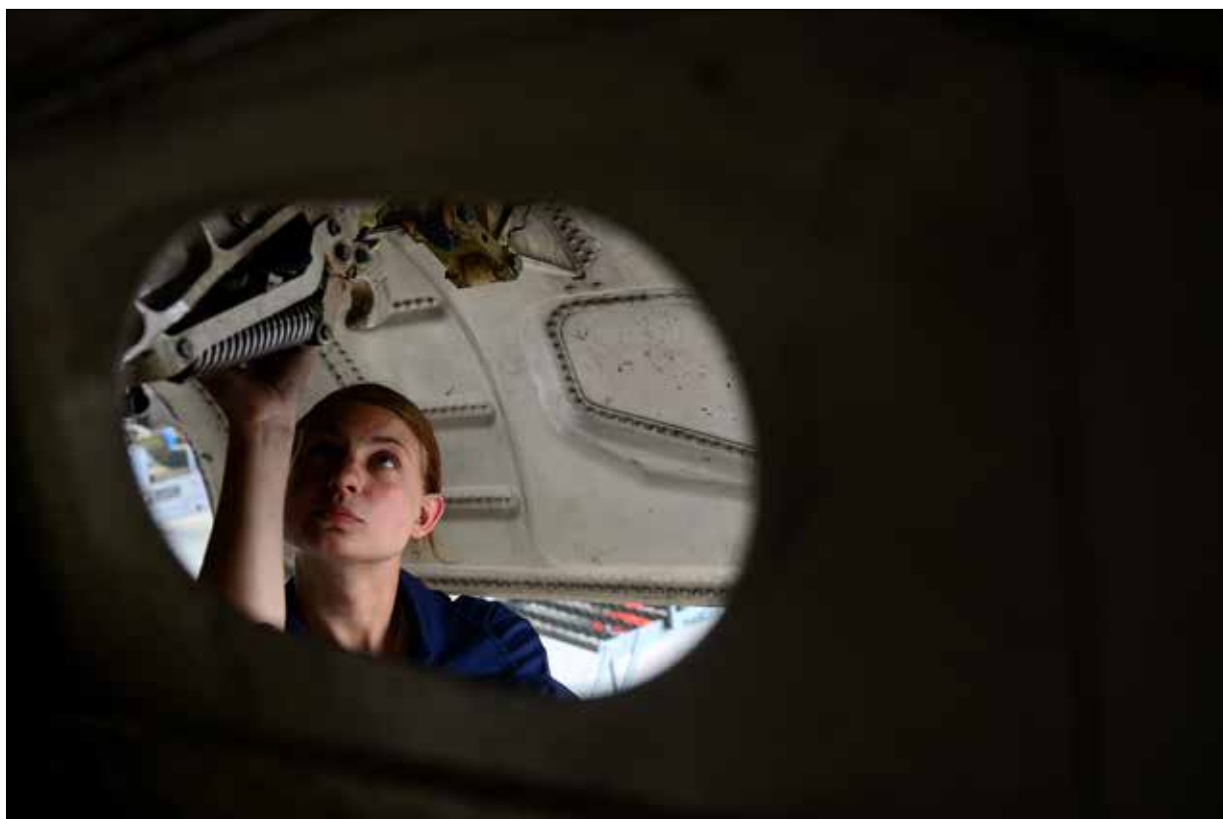
Staff Sgt. Elizabeth Dietrick, 8th Maintenance Squadron inspection section team member, inspects the landing gear of an F-16 Fighting Falcon at Kunsan Air Base, Republic of Korea, June 9, 2015. Dietrick works with a team of Airmen during phase inspections to take an in-depth look at aircraft before and after flight. Phase inspections are performed on aircraft every 400 flight hours and involve procedural maintenance actions that require robust attention to detail. (U.S. Air Force photos by Staff Sgt. Nick Wilson)
