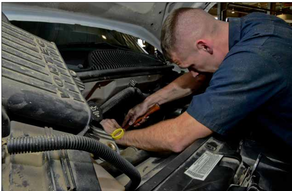
(Left) Senior Airman Justin Morris, 51st Logistics Readiness Squadron vehicle maintainer, installs an alternator in a van on Osan Air Base, Republic of Korea, Sept. 1, 2015. Vehicle maintenance technicians learn to maintain and repair more than 60 different types of government-vehicles operated on and off base. (U.S. Air Force photos by Senior Airman Kristin High)
