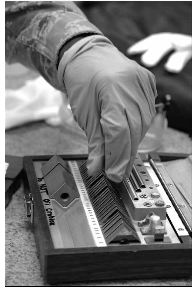
Airman 1st Class Marques Johnson, 51st Maintenance Squadron precision measurement equipment laboratory technician, puts away gauge blocks in the new PMEL facility on Osan Air Base, Republic of Korea. Gauge blocks are used to measure a series of comparisons and are at least four times more accurate than the unit being tested.
