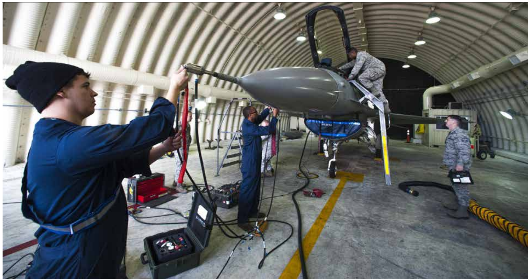
Senior Airman Jacob Clark, 8th Maintenance Squadron aircraft fuels systems journeyman, inspects an F-16 Fighting Falcon at Kunsan Air Base, Republic of Korea, Oct. 29, 2015. The fuels section is responsible for inspecting and repairing aircraft fuel systems, in-flight refueling receptacle systems, and other related components across F-16 aircraft. (U.S. Air Force photo by Staff Sgt. Nick Wilson)
