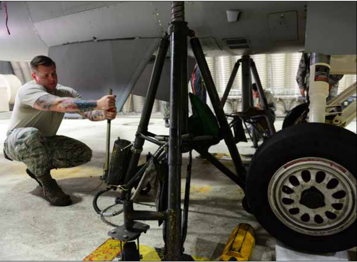
Staff Sgt. James McFadden, 35th Maintenance Group quality assurance manager, positions an aircraft jack beneath the wing of an F-16 Fighting Falcon during a weight and balance check class at Osan Air Base, Republic of Korea, Oct. 14, 2015. The class trained ROK and U.S. quality assurance managers how to properly weigh and balance aircraft using specialized systems. (U.S. Air Force photo by Staff Sgt. Amber Grimm)
