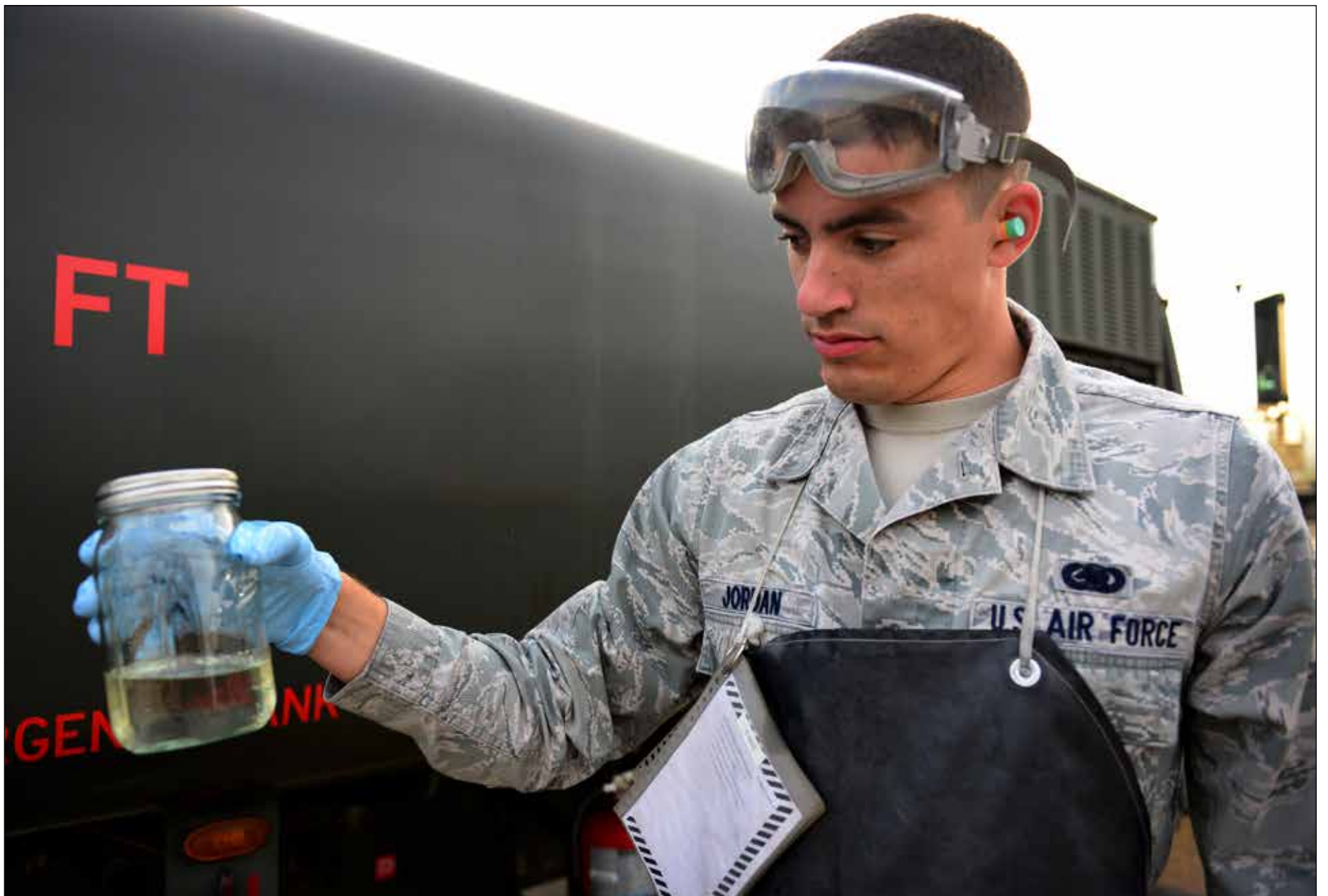
Senior Airman Joshua Jordan, 51st Logistics Readiness Squadron preventive maintenance technician, displays a sample jar of JP-8 jet fuel taken from one of the R-11 mobile fuel truck at Osan Air Base, Republic of Korea, Oct. 15, 2015. Daily samples are taken from each truck to test the fuel for excess water and contaminants. (U.S. Air Force photos by Staff Sgt. Amber Grimm)
