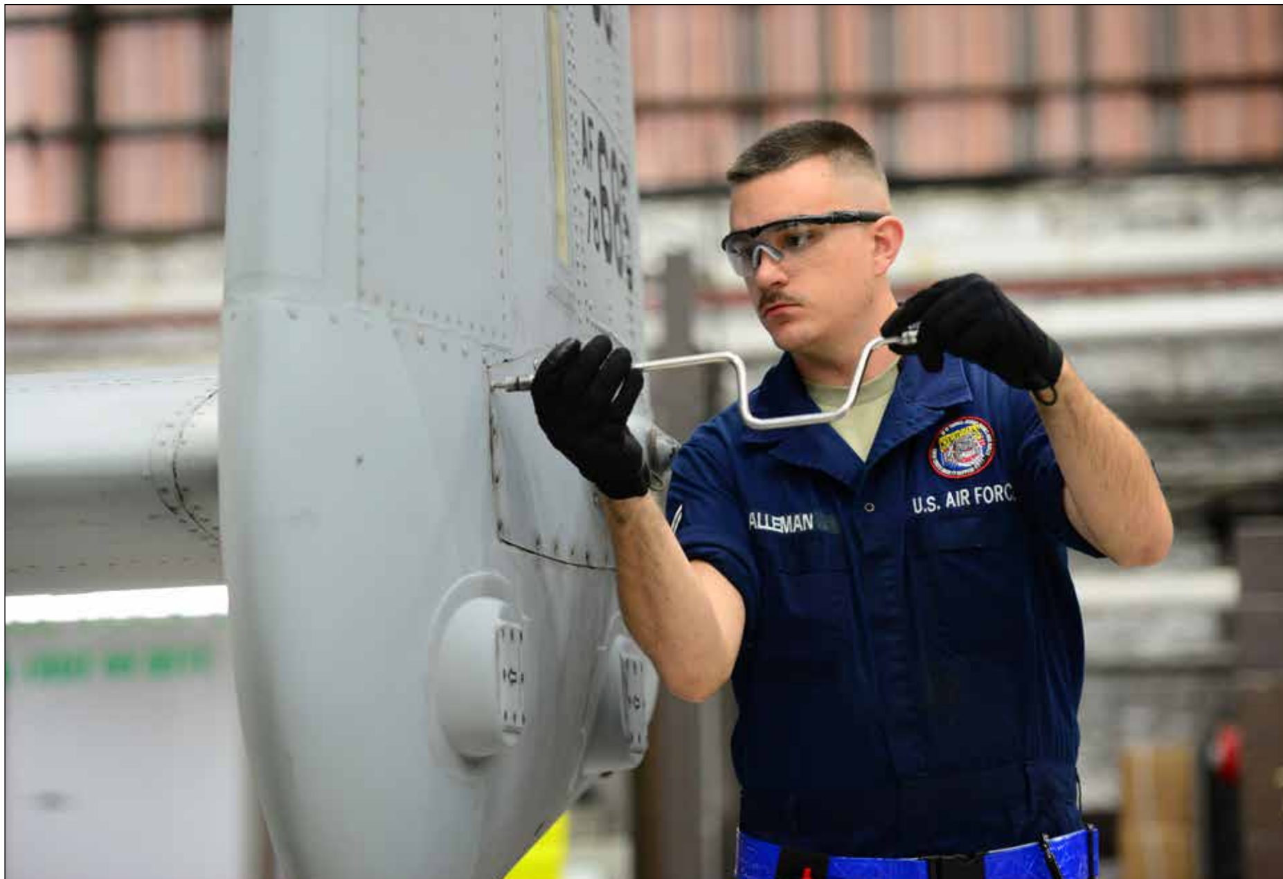
Airman 1st Class Cody Alleman, 51st Maintenance Squadron phase dock crew chief, removes screws from a tail panel on an A-10 Thunderbolt II during a routine phase inspection at Osan Air Base, Republic of Korea, Nov. 16, 2015. Panel removal is the first step in the in-depth inspection and preventive maintenance regiment the airframe must undergo after every 500 flight hours. (U.S. Air Force photos by Staff Sgt. Amber Grimm)
