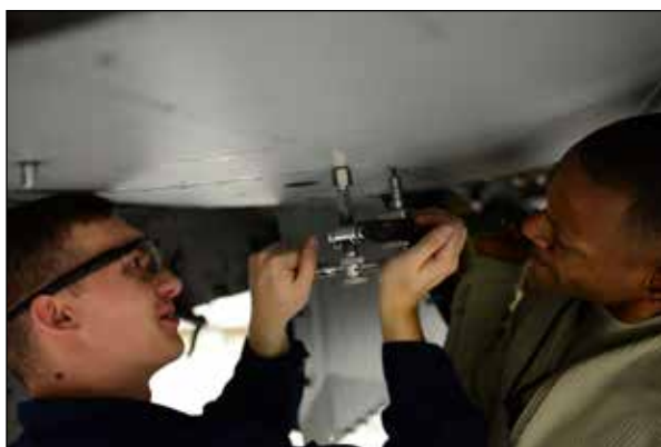
Tech. Sgt. Justin Archer and Airman 1st Class Cody Velloff, 51st Maintenance Squadron phase dock crew chiefs, work together to remove screws from a panel on the belly of an A-10 Thunderbolt II during a routine phase inspection at Osan Air Base, Republic of Korea, Nov. 16, 2015. Panel removal is the first step in the in-depth inspection and preventive maintenance regiment the airframe must undergo after every 500 flight hours.
