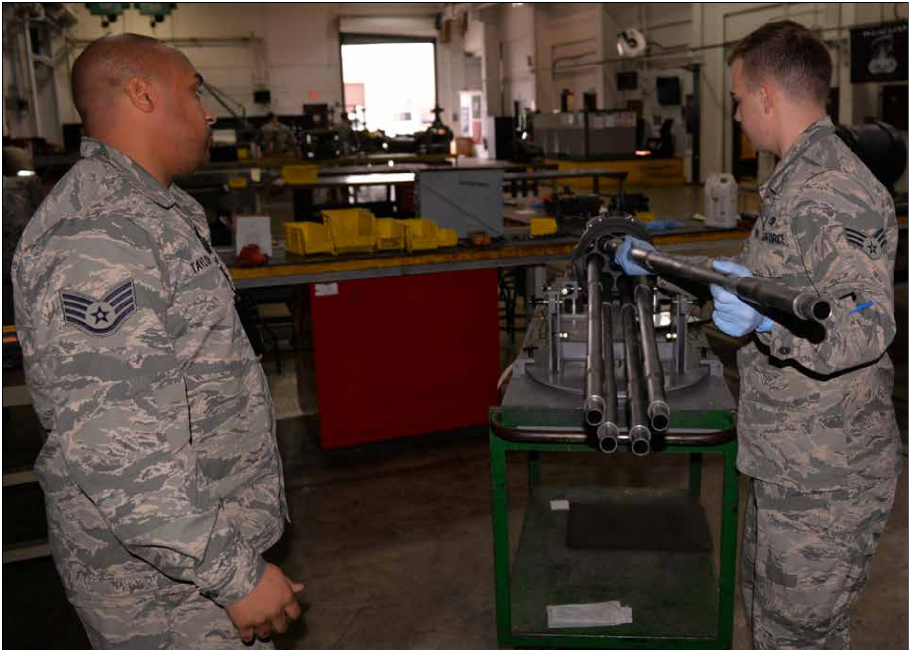
Staff Sgt. Robert Taylor, 51st Munitions Squadron F-16 armament floor chief, and Senior Airman Jacob Brown, 51st MUNS aircraft armament systems journeyman, put a 20-mm gun for an F-16 Fighting Falcon back together after performing maintenance Nov. 18, 2015, at Osan Air Base, Republic of Korea. These maintainers from the 51st MUNS armament flight keep the F-16 Fighting Falcon weapon systems operational both day and night. (U.S. Air Force photo by Staff Sgt. Benjamin Sutton) (Editor's note: A part of this image was blacked out for operational security reasons.)
