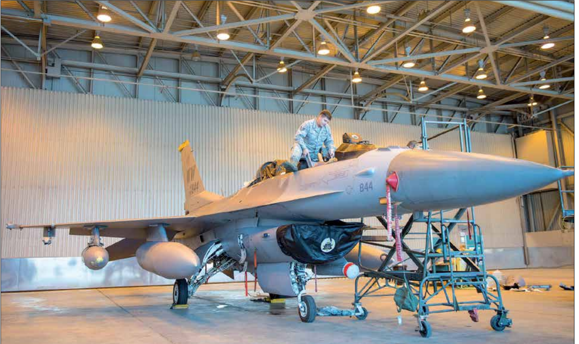
U.S. Air Force Staff Sgt. Corey Holt, an aircrew egress systems craftsman assigned to the 35th Maintenance Squadron, Misawa Air Base (AB), Japan, holds an ejection seat still in an F-16D Fighting Falcon aircraft while Staff Sgt. Shawn Layou, an aircrew egress systems craftsman assigned to the 8th Maintenance Squadron, Kunsan AB, Republic of Korea, bolts it into place Aug. 9, 2016, during RED FLAG-Alaska (RF-A) 16-3 at Eielson Air Force Base, Alaska. Units from across the Department of Defense and partner nations send units to Eielson for RF-A to train for contingency operations in a controlled environment stressing joint and multinational integration. (U.S. Air Force photo by Staff Sgt. Shawn Nickel)
