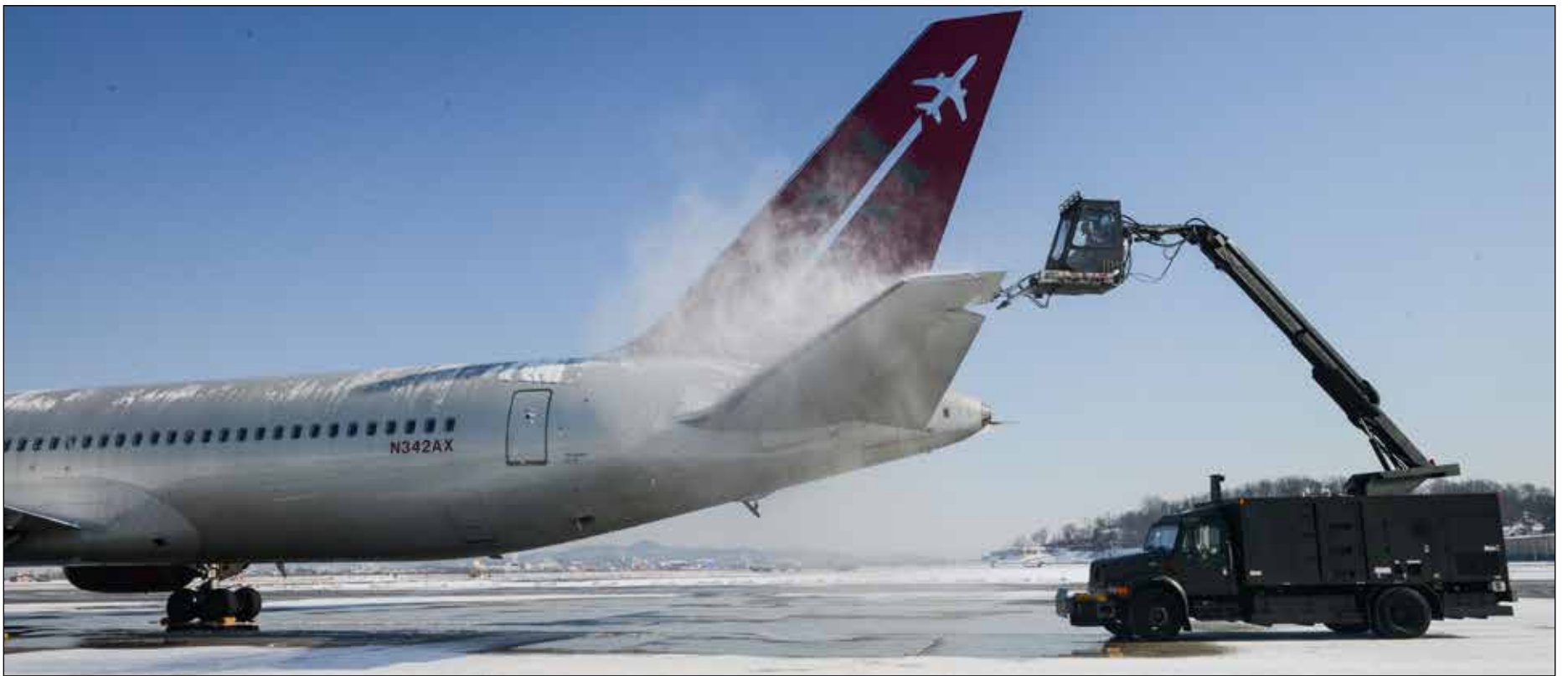
An Airman from the 51st Maintenance Squadron uses an aircraft de-icer on the Patriot Express passenger aircraft after a large amount of snowfall at Osan Air Base, Republic of Korea, Jan. 14, 2016. The de-icing process ensures the safe travel of passengers and cargo. (U.S. Air Force photos by Airman 1st Class Dillian Bamman)
