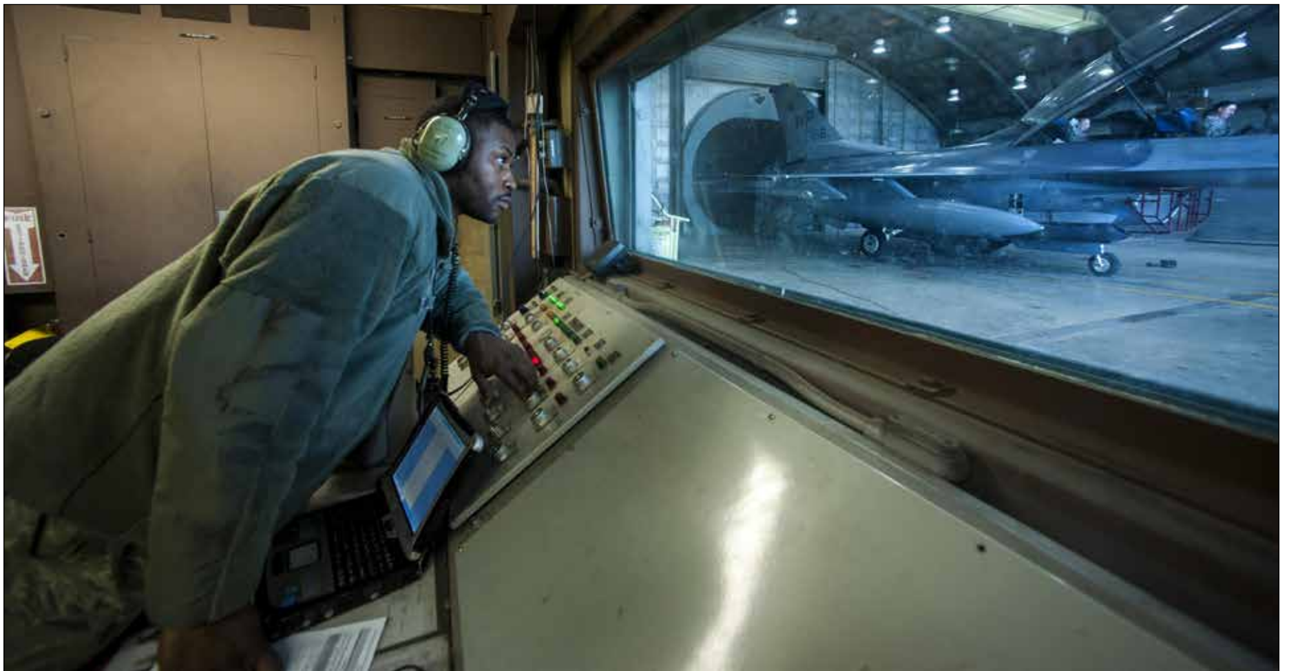
Tech. Sgt. Rowland Thagard, 8th Maintenance Squadron assistant propulsion section chief, oversees Airmen during an engine test in a hush house at Kunsan Air Base, Republic of Korea, Dec. 9, 2015. In addition to the hush house, the 8th MXS maintenance flight encompasses multiple duty sections, which include a tire shop, aerospace propulsion, crash damage, aircraft recovery and phase. (U.S. Air Force photos by Staff Sgt. Nick Wilson)
