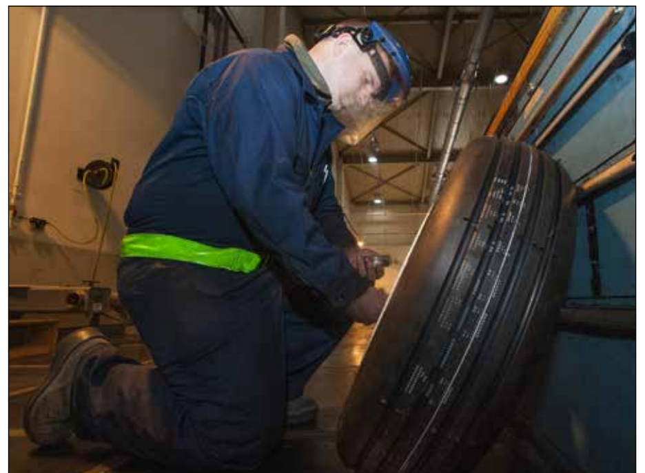
Senior Airman Matthew Ring, 8th Maintenance Squadron transient assistance crash recovery journeyman, signs a tag after performing a leak check on an F-16 Fighting Falcon landing gear tire at Kunsan Air Base, Republic of Korea, Jan. 7, 2016. In the tire shop, one of Ring's responsibilities is to ensure that he gets tires from the aircraft maintenance units, breaks them down, rebuilds them and get them returned as soon as possible.
