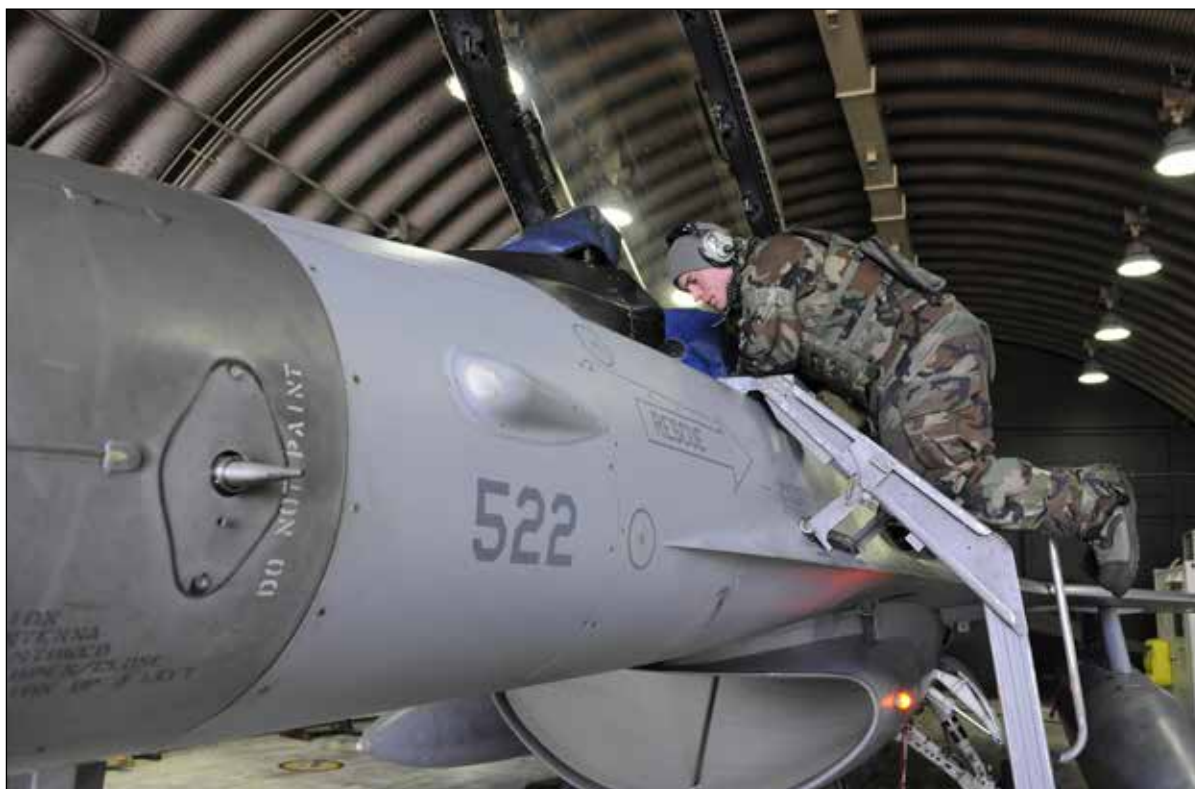
(Left) Senior Airman Kollin Bell, 35th Aircraft Maintenance Squadron crew chief, conducts a pre-flight lights inspection to ensure all critical lights are working on an F-16 Fighting Falcon during Beverly Pack 16-2 at Kunsan Air Base, Republic of Korea, Feb. 3, 2015. The 8th Maintenance Group's over 1,000 Airmen have worked around-the-clock amid temperatures in the teens to ensure all the wing's F-16s are ready to fly safely.
