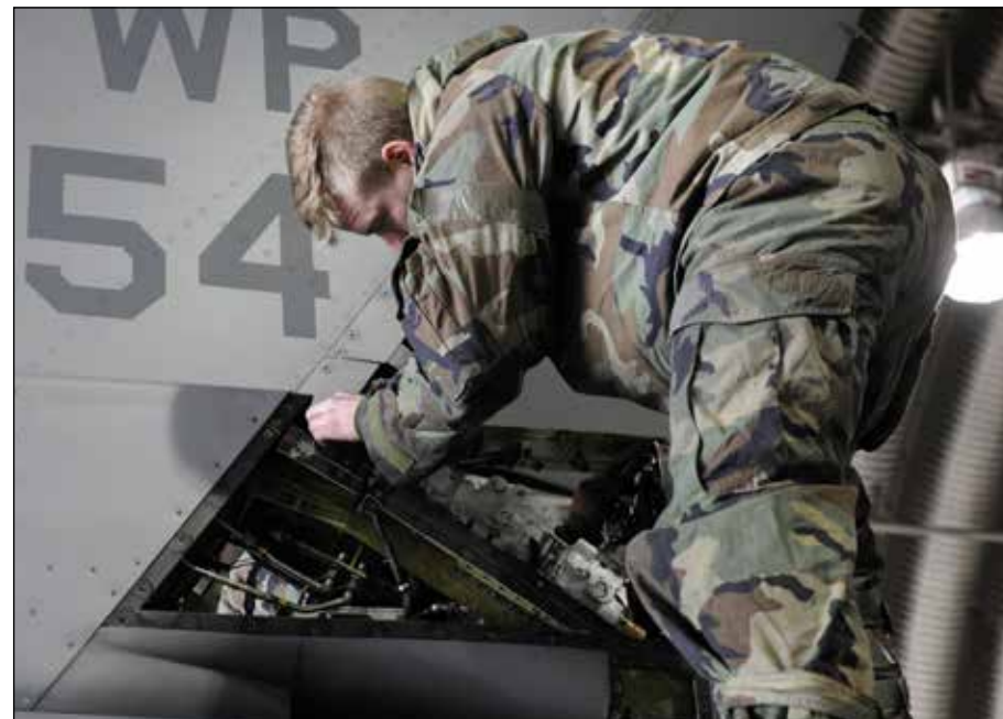
Staff Sgt. Brandon Rachuy, 80th Aircraft Maintenance Squadron dedicated crew chief, works on removing a rudder servo actuator on an F-16 Fighting Falcon during Beverly Pack 16-2 at Kunsan Air Base, Republic of Korea, Feb. 3, 2015. Airmen work around the clock no matter the conditions during the exercises here on Kunsan.
