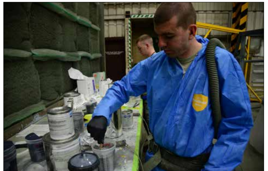
Senior Airman Matthew Cook, 51st Maintenance Squadron aircraft structural maintainer, mixes a container of advanced protective paint at Osan Air Base, Republic of Korea, Jan. 6, 2016. The paint is used to touch up scratches and chips in existing coating and prevents corrosion from developing in the metal.
