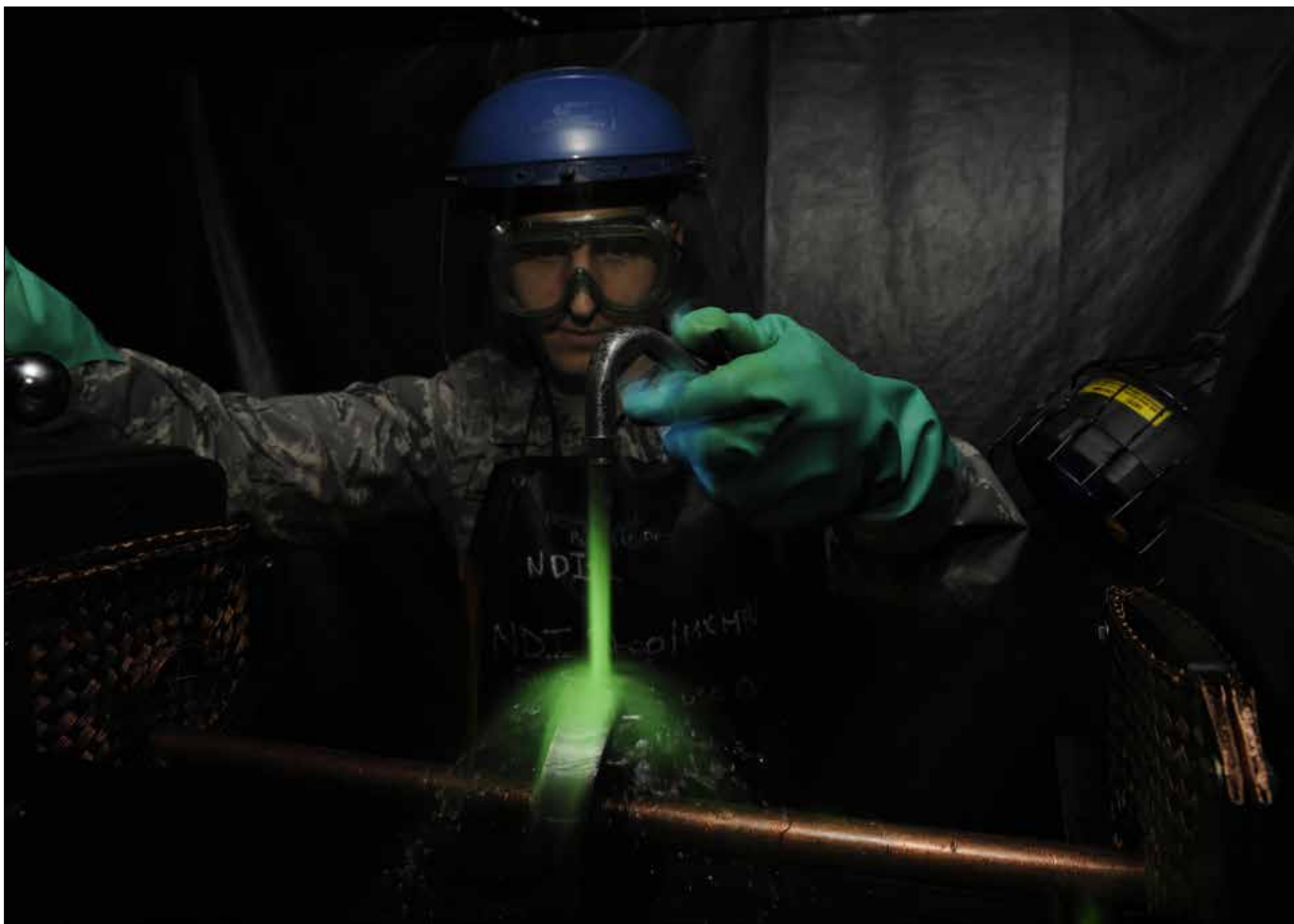
Staff Sgt. John Stevens, 8th Maintenance Squadron non-destructive inspection shift supervisor, uses ultraviolet lights to inspect aircraft parts March 2, 2016, at Kunsan Air Base, Republic of Korea. The 8th MXS NDI shop inspects metal objects ranging from nuts and bolts, to large hooks and sheets of metal to ensure the safety of the aircraft. (U.S. Air Force photos by Senior Airman Dustin King)
