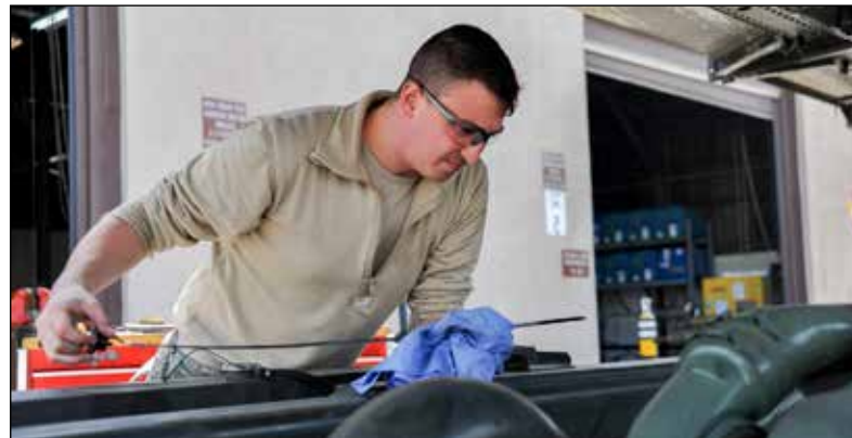
(Above) Senior Airman Jonathan Rowley, 51st Logistics Readiness Squadron sorting generating and aircraft sustaining vehicle maintainer, checks oil on a Tunner 60K loader at Osan Air Base, Republic of Korea, March 30, 2016. The loader can transport six pallets of cargo for loading on commercial and military cargo aircraft. (Right) Prepares to conduct a limited technical inspection on Tunner 60K loader at Osan Air Base, Republic of Korea, March 30, 2016. The inspection consisted of operational function checks on the mechanical, electrical and hydraulic systems.
