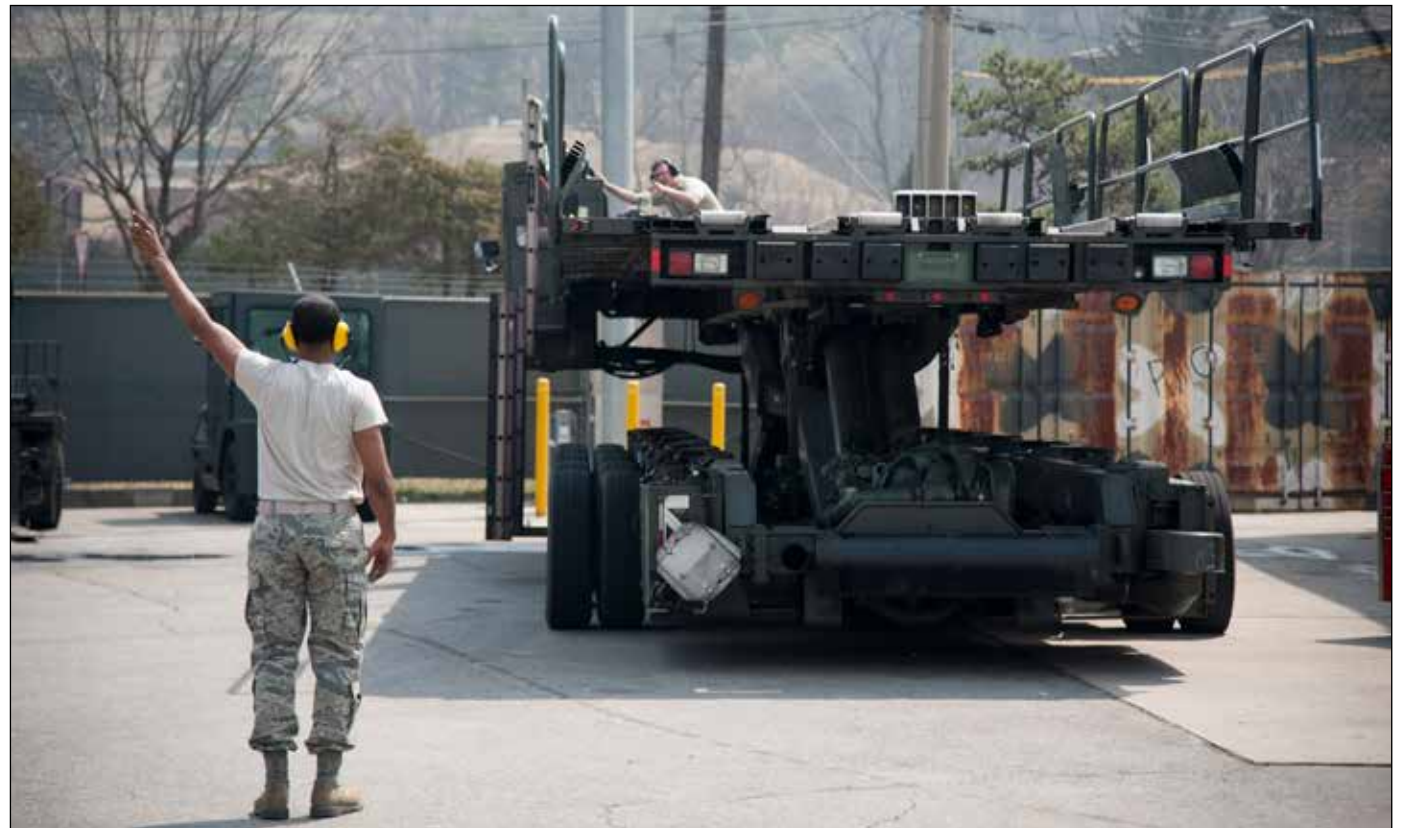
Staff Sgt. Sergio McLaughlin, 51st Logistics Readiness Squadron sorting generating and aircraft sustaining vehicle maintainer, checks turn signals for serviceability on a Tunner 60K loader at Osan Air Base, Republic of Korea, March 30, 2016. The loader can transport six pallets of cargo for loading on commercial and military cargo aircraft. (U.S. Air Force photos by Staff Sgt. Jonathan Steffen)
