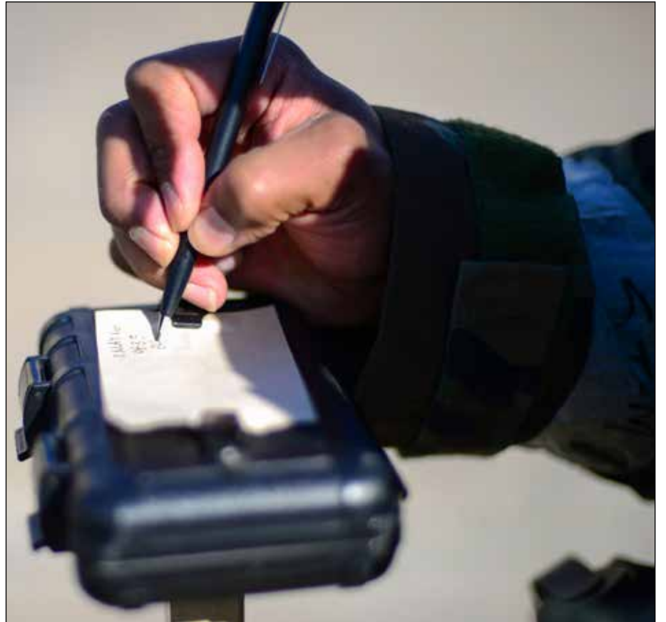
A 51st Civil Engineer Squadron Airman marks a piece of M8 Chemical Detection Paper during a training exercise at Osan Air Base, Republic of Korea, May 11, 2016. The Airmen used the M8 paper to detect the presence of liquid, nerve and blister chemical agents after a simulated attack on the base, and is marked to ensure each piece can be properly documented for identification purposes. (U.S. Air Force photos by Senior Airman Victor J. Caputo)
