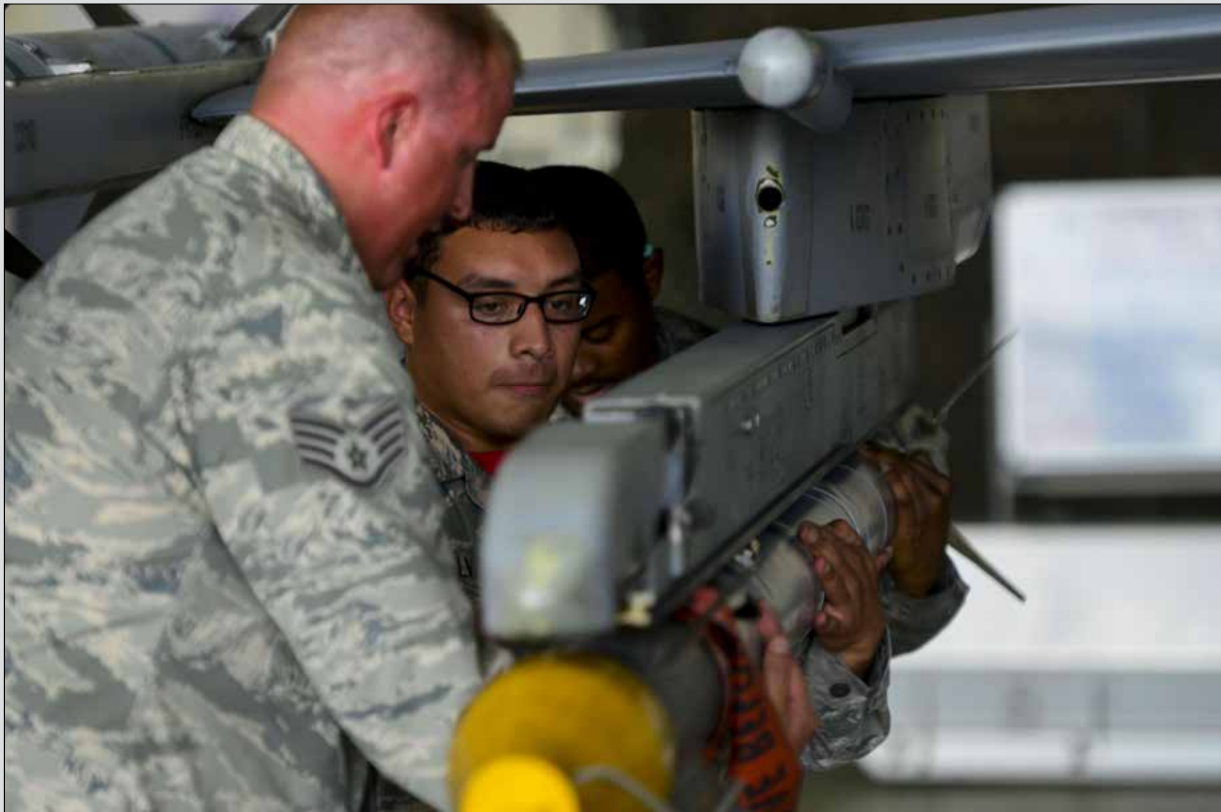
The 36th Aircraft Maintenance Unit weapons load crew team fastens an AIM-9 Sidewinder missile to an F-16 Fighting Falcon during the 51st Maintenance Group Weapons Load Crew of the Quarter competition at Osan Air Base, Republic of Korea, July 7, 2016. Weapons load teams from the 25th and 36th AMUs competed in dress and appearance, timing and technical order proficiency during the event. (U.S. Air Force photos by Senior Airman Victor J. Caputo)
