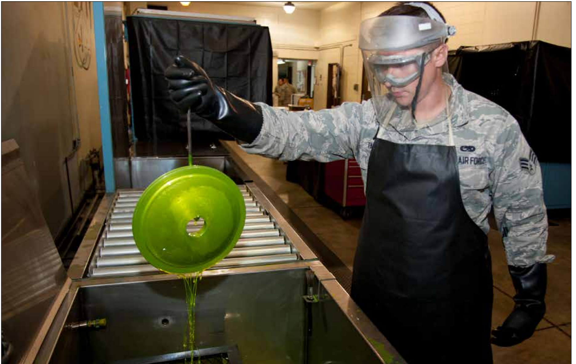
Senior Airman Nathan Talamantez, 51st Maintenance Squadron non-destructive inspection journeyman, pulls out a brake housing covered in fluorescent oil penetrant at Osan Air Base, Republic of Korea, June 28, 2016. Talamantez will use fluorescent oil penetrant to identify cracks in aircraft parts. Talamantez is assigned to the non-destructive inspection shop and is part of the fabrication flight which also has structural maintenance shop and metals technology. Fabrication flight Airmen identify, repair and build parts to working order so that Osan airframes are ready to fight tonight. (U.S. Air Force photos by Staff Sgt. Jonathan Steffen)
