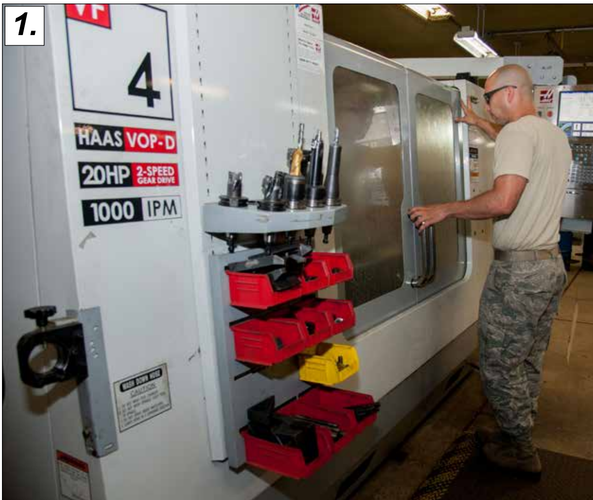
1. Tech. Sgt. Jesse Mcleod, 51st Maintenance Squadron aircrafts metals technology craftsman, operates a computer numeric control machine at Osan Air Base, Republic of Korea, June 28, 2016. The CNC machine is designed to make custom aircraft parts. Mcleod is assigned to the metals technology shop and is part of the fabrication flight, which also has non-destructive inspection and structural maintenance.
