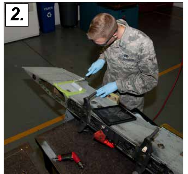
Senior Airman Nathan Talamantez, 51st Maintenance Squadron non-destructive inspection journeyman, pulls out a brake housing covered in fluorescent oil penetrant at Osan Air Base, Republic of Korea, June 28, 2016. Talamantez will use fluorescent oil penetrant to identify cracks in aircraft parts. Talamantez is assigned to the non-destructive inspection shop and is part of the fabrication flight which also has structural maintenance shop and metals technology. Fabrication flight Airmen identify, repair and build parts to working order so that Osan airframes are ready to fight tonight. (U.S. Air Force photos by Staff Sgt. Jonathan Steffen)
