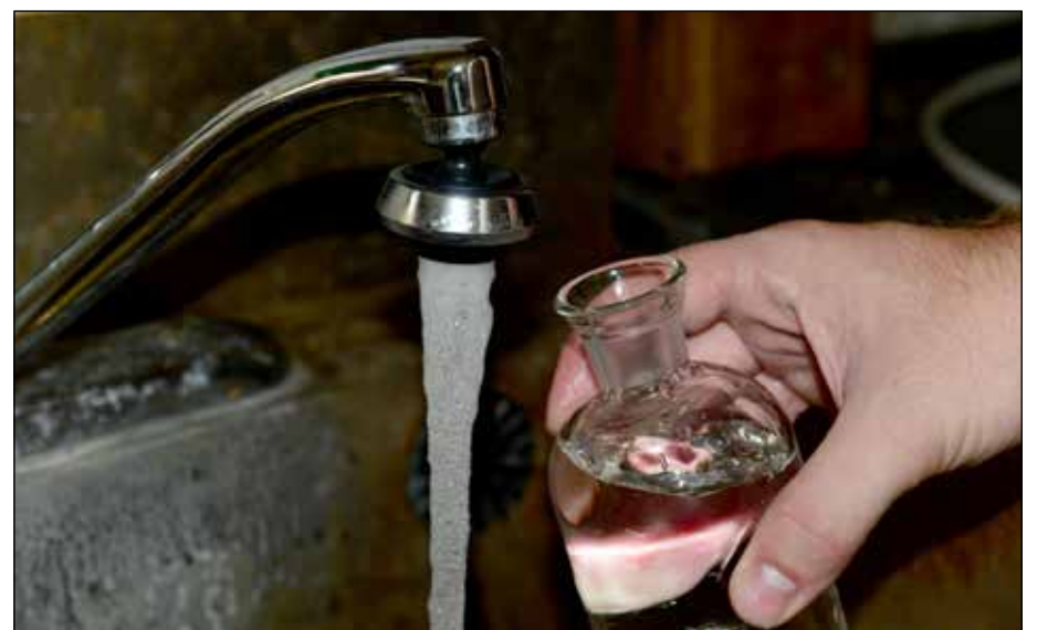
U.S. Air Force Senior Airman Jeremy Robinson, 8th Civil Engineer Squadron Water and Fuels system technician, gathers a sample of the first place water runs out of the facility for pH level test at Kunsan Air Base, Republic of Korea, Aug. 24, 2016. 8th CES Airmen monitor city water on a bi-hourly basis and add additional chlorine to the water to ensure every facility on base has water that is safe to drink.
