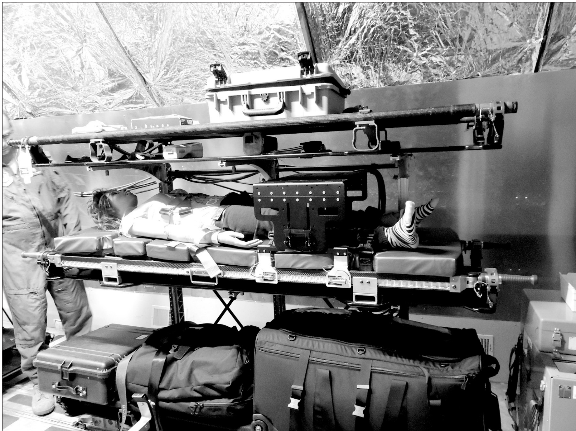
Cornerstone Research Group's aeromedical evacuation stretcher is shown during a compatibility test on a KC-135 Stratotanker. (Courtesy photo by Cornerstone Research Group)
