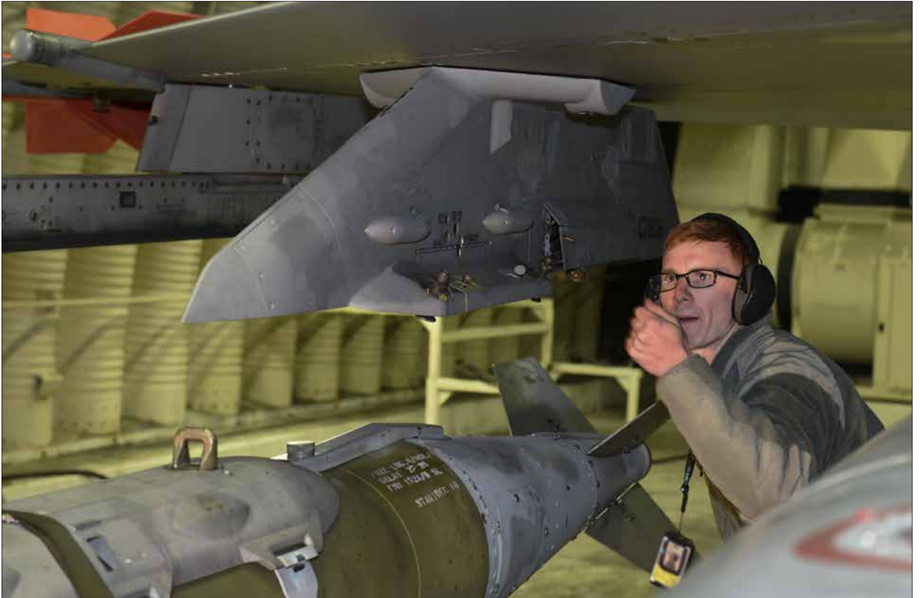
Staff Sgt. Kenneth Gullette, 35th Aircraft Maintenance Unit weapons load crew chief, guides a Joint Direct Attack Munition GBU-31 onto the wing of an F-16 Fighting Falcon at Kunsan Air Base, Republic of Korea, Nov. 30, 2016. Members of the 35th AMU safely prepare F-16's for a variety of missions, which feed into the 8th Fighter Wings priorities of defending the base and being postured to respond to any threats. (U.S. Air Force photo by Senior Airman Michael Hunsaker)
