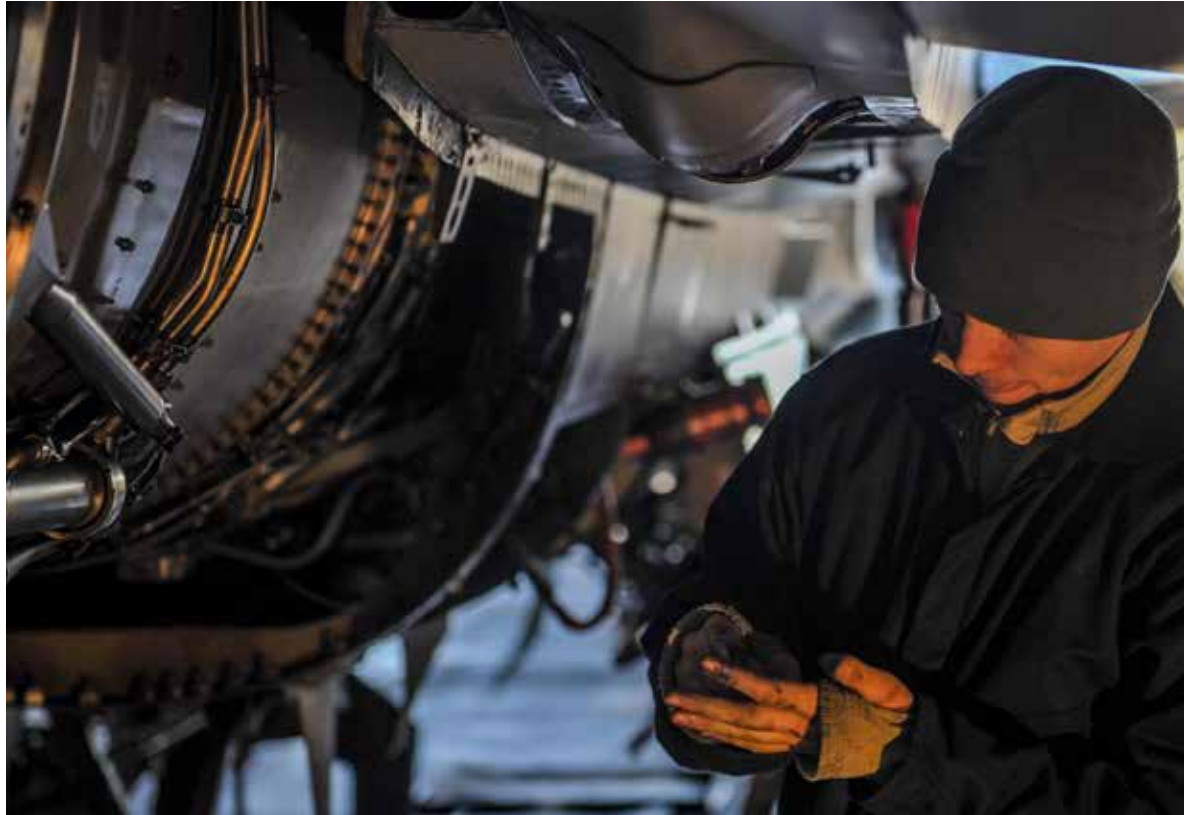
Senior Airman Shane Fortune, 8th Maintenance Squadron phase inspection team member, inspects a part of an F-16 Fighting Falcon at Kunsan Air Base, Republic of Korea, Dec. 6, 2016. Fortune works with a team of Airmen during phase inspections to ensure aircraft are prepared for flight. Phase inspections are performed on aircraft every 400 flight hours and involve procedural maintenance actions that require robust attention to detail. (U.S. Air Force photo by Senior Airman Colville McFee)
