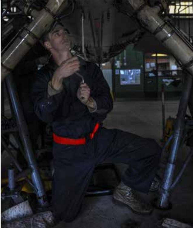
Airman 1st Class Alec Eckert, 8th Maintenance Squadron inspection section team member, screws panels into an F-16 Fighting Falcon at Kunsan Air Base, Republic of Korea, Dec. 6, 2016. Phase inspections are performed on aircraft every 400 flight hours and involve procedural maintenance actions that require robust attention to detail. (U.S. Air Force photo by Senior Airman Colville McFee)
