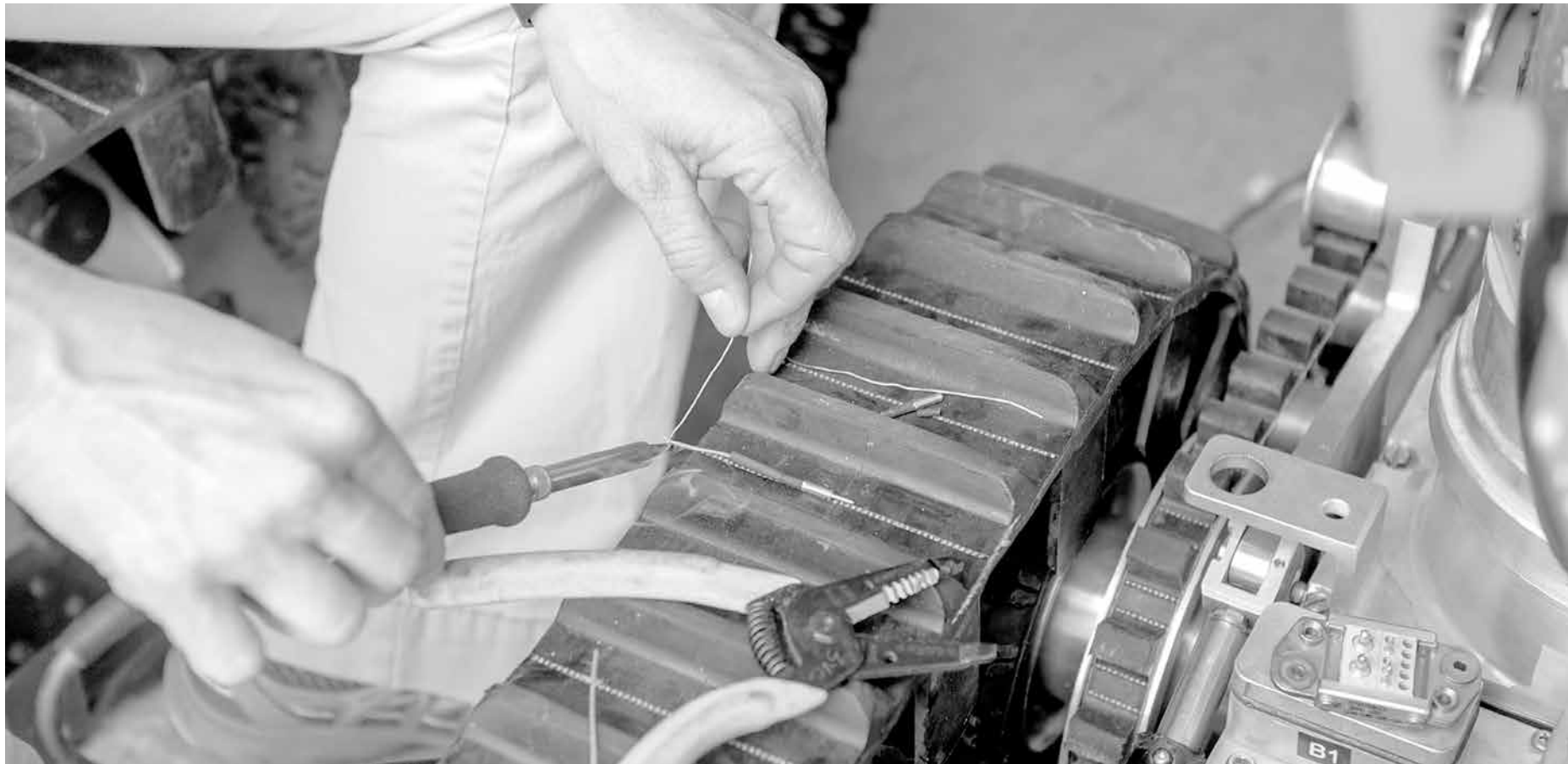
Kimberly Tipton, Remotec instructor, replaces the pin of a connector on an Air Force Medium Sized Robot at Kunsan Air Base, Republic of Korea, Aug. 10, 2017. While only weighing 223 pounds, the AFMSR can lift objects up to 125 pounds. (U.S. Air Force photo by Senior Airman Colby L. Hardin)
