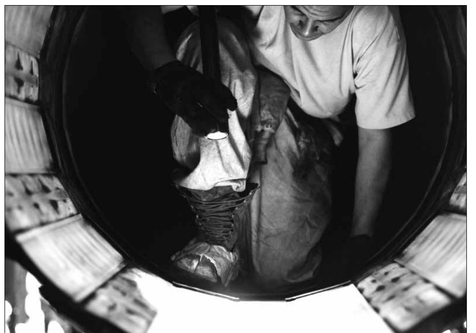
<Bottom> U.S. Air Force Tech. Sgt. Kenneth Arlequin, 51st Maintenance Squadron aerospace propulsion craftsman, performs an intake and exhaust inspection on an F-16 Fighting Falcon aircraft in the Phase Hangar at Osan Air Base, Republic of Korea on Aug. 28, 2017. From engines and egress to corrosion control and sheet metal, every maintenance agency on the flightline has a hand in the phase maintenance, bringing the specialists straight to the jet for the inspection and refurbish. (U.S. Air Force photo by Staff Sgt. Alex Fox Echols III)
