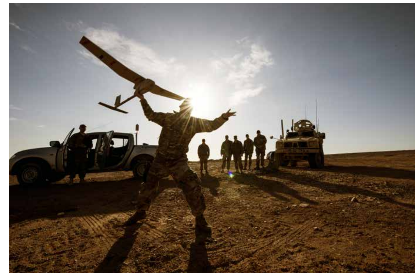
T ech Sgt. Matthew Coutts, assigned to the 332d Expeditionary Security Forces Squadron, launches a Raven B Digital Data Link drone during a demonstration Jan. 24, 2018 in Southwest Asia. After takeoff, the Raven B uses battery power to patrol the air for 60-90 minutes at a time. (U.S. Air Force photo by Staff Sgt. Joshua Kleinholz)
