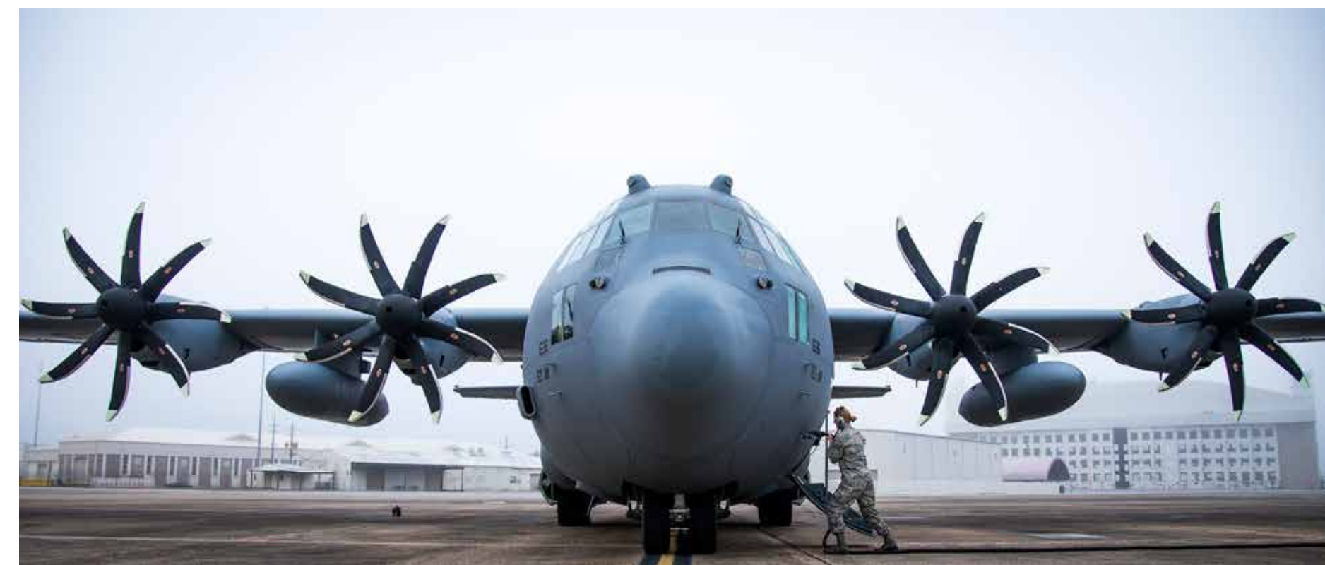
A 153rd Airlift Wing maintainer plugs in a generator cable into her C-130H Hercules after arriving at Eglin Air Force Base, Fla., Jan. 11, 2018. The Air Force's first fully upgraded C-130H is here for test and evaluation on its new modified propeller system and engines. (U.S. Air Force photo by Samuel King Jr.)
