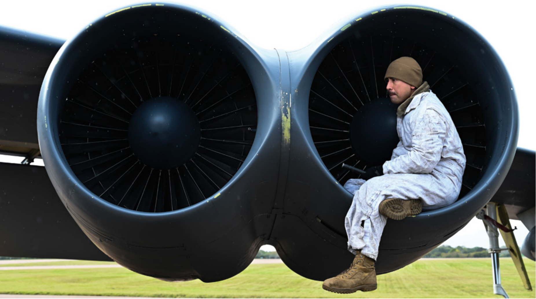
S taff Sgt. Stephen Zbinovec, 2nd Aircraft Maintenance Squadron, 96th Aircraft Maintenance Unit crew chief, inspects the engine of a U.S. Air Force B-52H Stratofortress at RAF Fairford, United Kingdom, Oct. 18, 2019. Airmen from the 2nd AMXS inspected the B-52 after it landed to ensure there was no damage and to prepare it for the next mission. (U.S. Air Force photo by Senior Airman Stuart Bright) ▲
