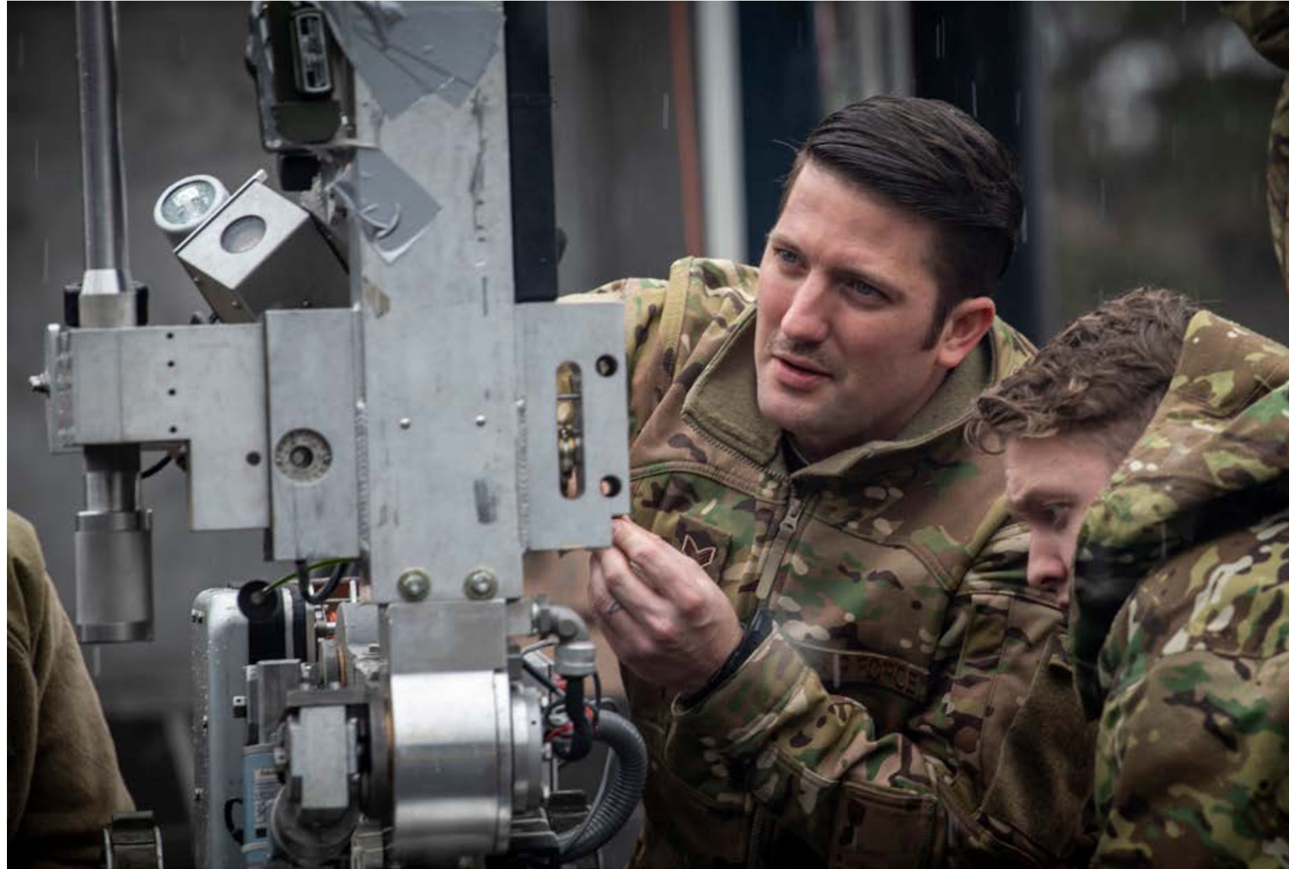
U.S. Air Force Senior Airman Tyrone Powell, left, a 35th Civil Engineer Squadron Explosive Ordnance Disposal journeyman and Airman 1st Class Derik Rosse, right, a 35th CES EOD apprentice, inspect an F6A robot at Misawa Air Base, Japan, March 3, 2020. Personnel work together with reconnaissance robots to help locate, disarm and remove improvised explosive devices. The robots enter inaccessible areas operated by the EOD team, mitigating the risk of danger during training. (U.S. Air Force photo by Airman 1st Class China M. Shock)
