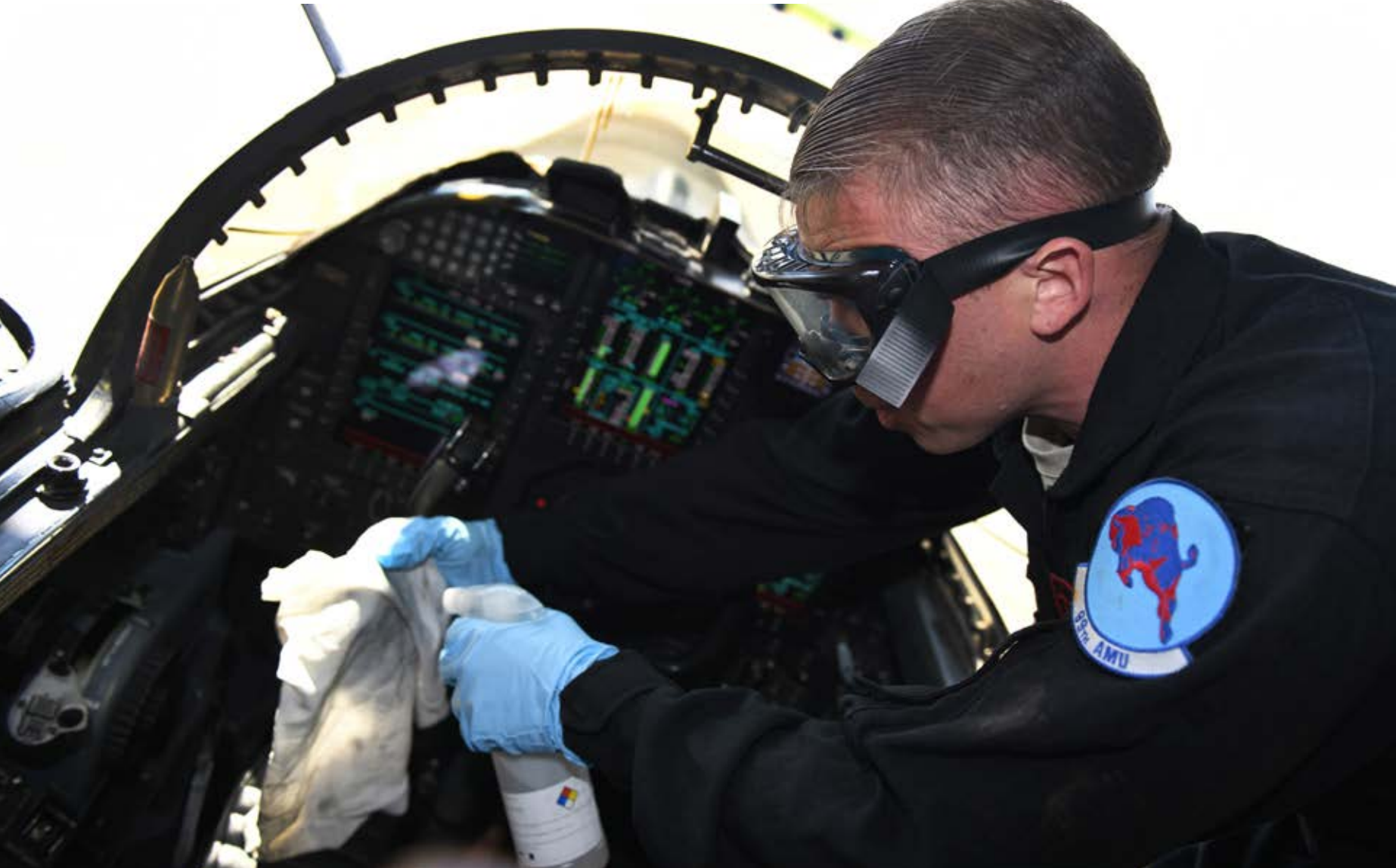
S taff Sgt. Brandon Green, 99th Aircraft Maintenance Unit dedicated crew chief, sprays disinfectant liquid on a rag to sanitize the cockpit of a U-2, March 23, 2020, at Beale Air Force Base, Calif. The cockpits on Beale AFB's fleet of U-2s are being sanitized on a regular basis to prevent the spread of COVID-19. (U.S. Air Force photo by Airman 1st Class Luis A. Ruiz-Vazquez) ▼
