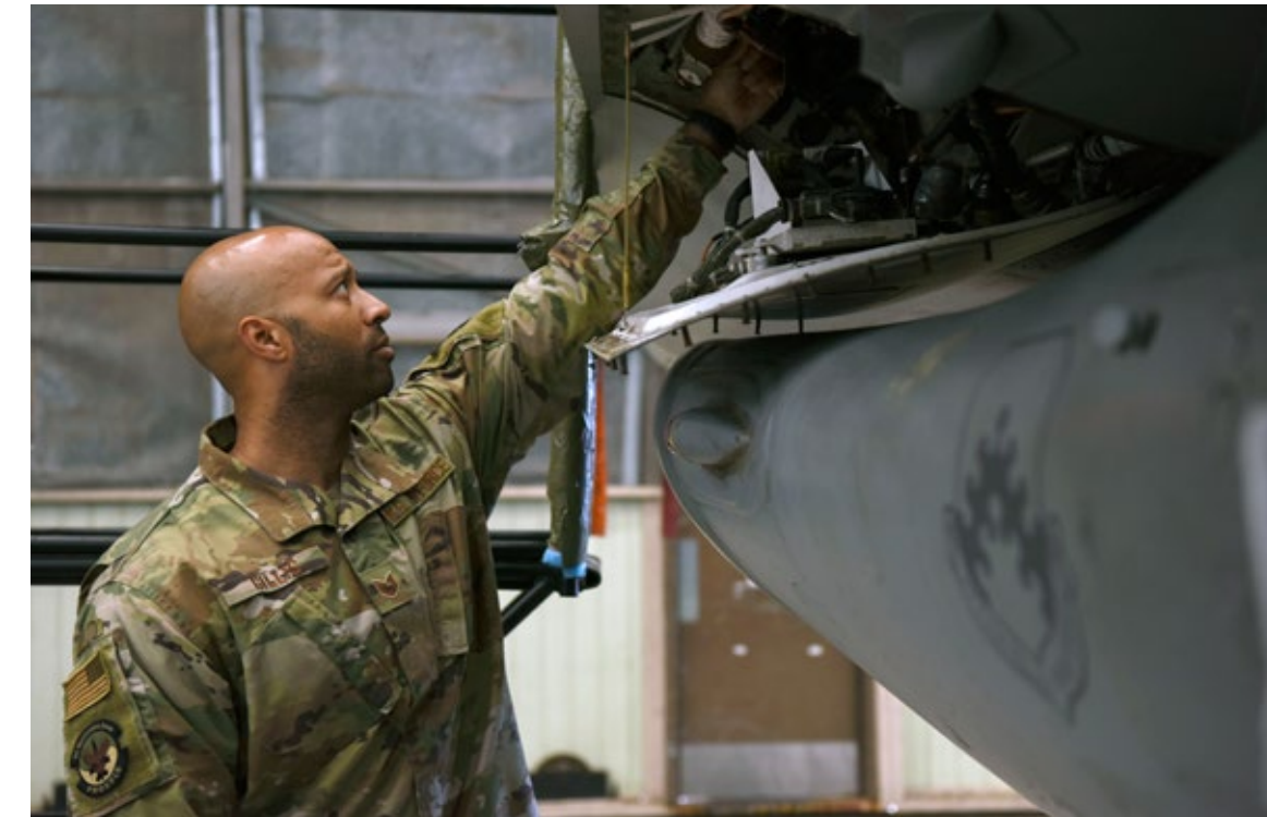
U.S. Air Force Tech. Sgt. Pierce Gillis, 8th Maintenance Group quality inspector, ensures an environmental control system duct cap is securely tightened at Kunsan Air Base, Republic of Korea, May 18, 2020. QA's primary mission is to inspect and ensure maintenance processes are being completed in accordance with Air Force Instructions to ensure the safety of all personnel. (U.S. Air Force photo by Senior Airman Jessica Blair)
