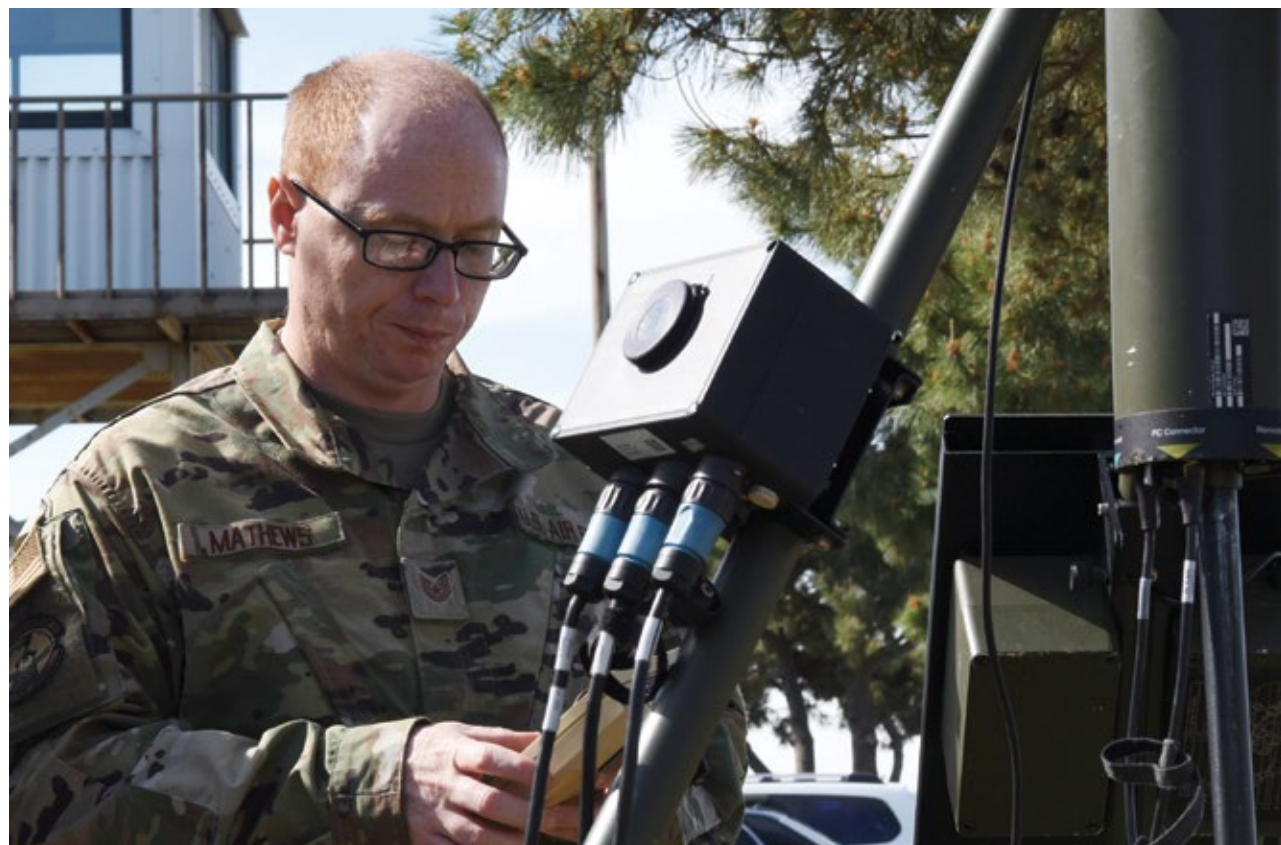
The TMQ-53 is a portable, automated weather station used to set up in austere locations to attain weather data from the area. The equipment takes roughly 30 minutes for a two-member team to set up and 45 minutes for a lone member. (U.S. Air Force photo by Staff Sgt. Anthony Hetlage)
