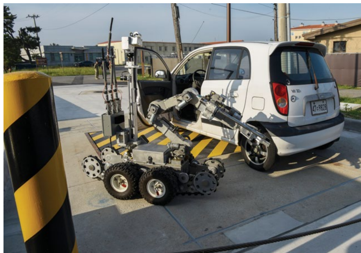
U.S. Air Force Senior Airman Jermy Hoban, 8th Civil Engineer Squadron explosive ordnance disposal team member, operates the EOD robot to open the vehicle's doors during routine training at Kunsan Air Base, Republic of Korea, May 27, 2020. Hoban remotely operated the robot to open all of the doors and inspect the vehicle for additional threats. (U.S. Air Force photo by Senior Airman Jessica Blair)+
