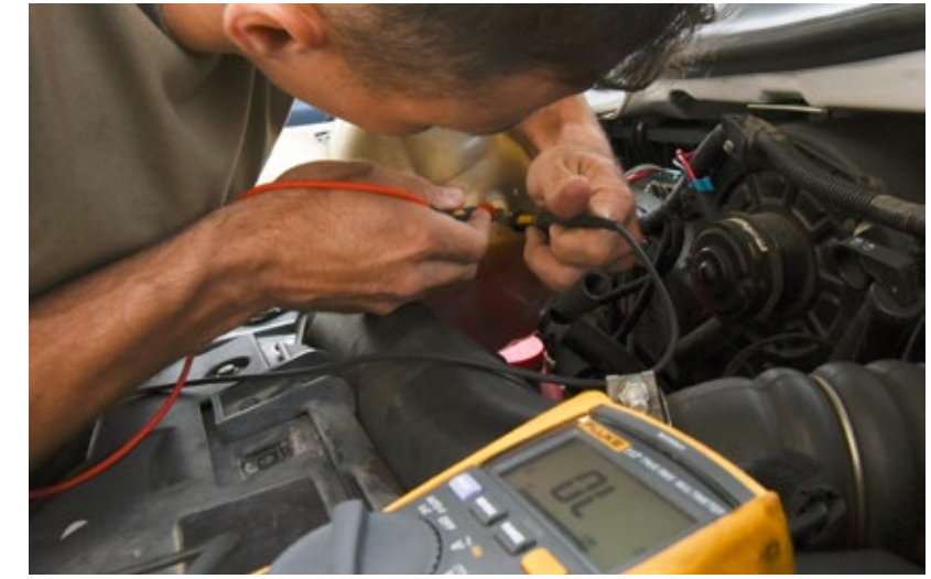
Tech. Sgt. John Bishop, 8th Logistics Readiness Squadron NCO in charge of vehicle maintenance, inspects a vehicle at Kunsan Air Base, Republic of Korea, June 4, 2020. Bishop is troubleshooting a low coolant light on the vehicle by checking the voltage to ensure the sensor is getting power. (U.S. Air Force photo by Staff Sgt. Anthony Hetlage) ◀
