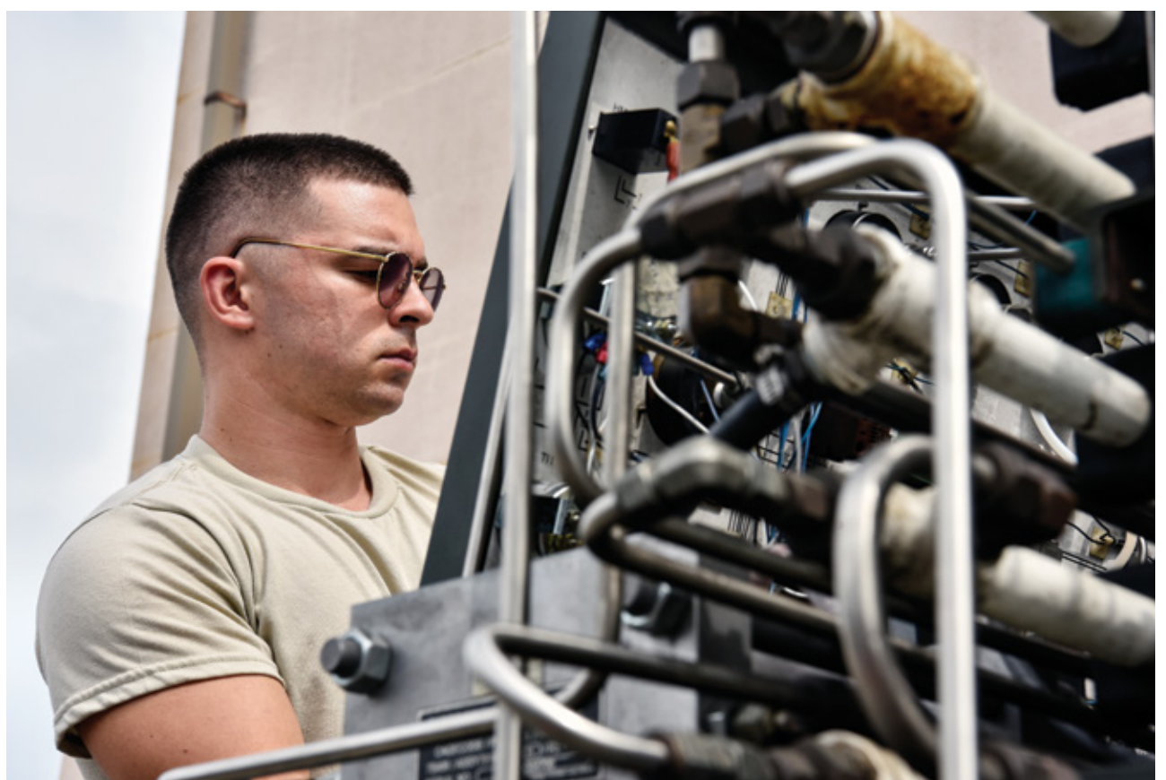
Senior Airman Nicholas Rapacon, 8th Maintenance Squadron Aerospace Ground Equipment flight journeyman, troubleshoots a Self-Generating Nitrogen Servicing Cart electrical system at Kunsan Air Base, Republic of Korea, Aug. 4, 2020. The SGNSC is a 3,000-pound, field support equipment designed to eliminate nitrogen resupply requirements specifically for the F-16 Fighting Falcon. (U.S. Air Force photo by Senior Airman Mya M. Crosby)
