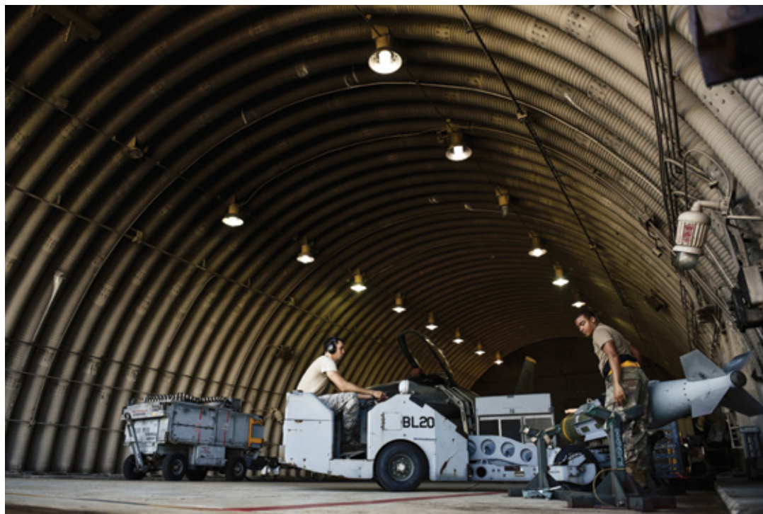
Staff Sgt. Trevor Glass and Senior Airman Fariq Islam, 80th Aircraft Maintenance Unit weapons armament systems specialists, prepare to mount a Joint Direct Attack Munition, or JDAM, onto an F-16 Fighting Falcon. Maintainers prepare aircraft for flight during routine training events. (U.S. Air Force photo by Senior Airman Mya M. Crosby) ▲
