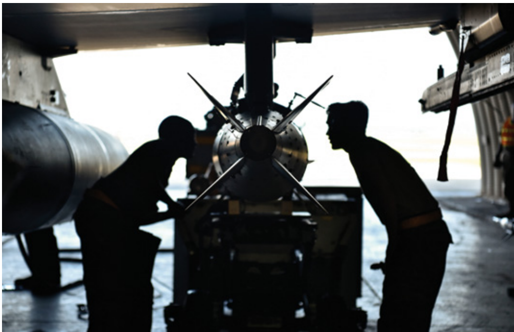
Staff Sgt. Trevor Glass and Airman Joseph Boik, 80th Aircraft Maintenance Unit armament systems specialists, secure a Joint Direct Attack Munition, or JDAM, onto an F-16 Fighting Falcon at Kunsan Air Base, Republic of Korea, Aug. 16, 2020. Maintainers prepare aircraft for flight during routine training events. (U.S. Air Force photo by Senior Airman Mya M. Crosby) ◀
