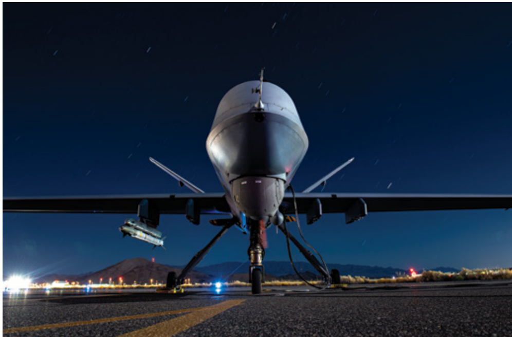
A MQ-9 Reaper, assigned to the 556th Test and Evaluation Squadron, armed with an AIM-9X missile sits on the flightline, Sept. 3, 2020, at Creech Air Force Base, Nev. The MQ-9 successfully employed a live air-to-air test of an AIM-9X Block 2 missile against a target BQM-167 drone simulating a cruise missile. (U.S. Air Force photo by Senior Airman Haley Stevens) ▼
