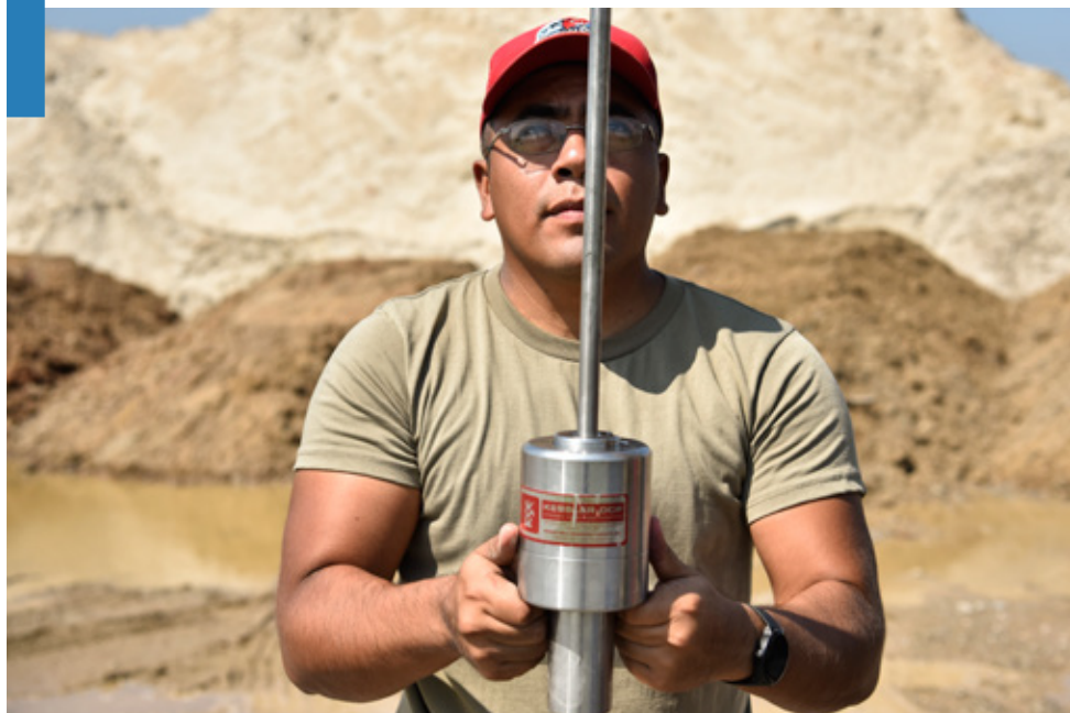
Master Sgt. David Carreon, assigned to the 554th RED HORSE, or Rapid Engineer Deployable Heavy Operational Repair Squadron Engineers, operates a dynamic cone penetrometer at Kunsan Air Base, Republic of Korea, Sept. 4, 2020. RED HORSE is self-sufficient, with rapid response capabilities, to conduct independent operations in remote, high-threat environments. (U.S. Air Force photo by Senior Airman Mya M. Crosby) ▲
