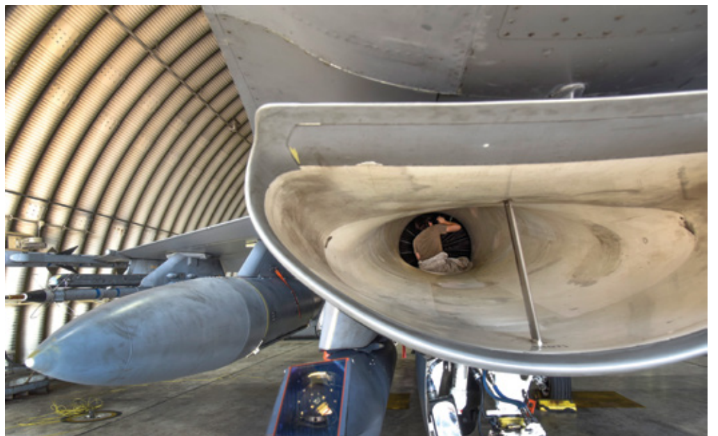
Staff Sgt. Abigail Backman, 80th Aircraft Maintenance Unit engines mechanic, inspects the exhaust of an F-16 Fighting Falcon on the flight line at Kunsan Air Base, Republic of Korea, Sept. 20, 2020. Aircraft intakes and exhausts are checked for foreign object debris and damage, both before and after flight. (U.S. Air Force photo by Staff Sgt. Kristin S. High) ▲ ▼
