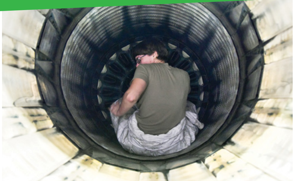
Staff Sgt. Abigail Backman, 80th Aircraft Maintenance Unit engines mechanic, inspects the exhaust of an F-16 Fighting Falcon on the flight line at Kunsan Air Base, Republic of Korea, Sept. 20, 2020. Aircraft intakes and exhausts are checked for foreign object debris and damage, both before and after flight. (U.S. Air Force photo by Staff Sgt. Kristin S. High) ▲ ▼
