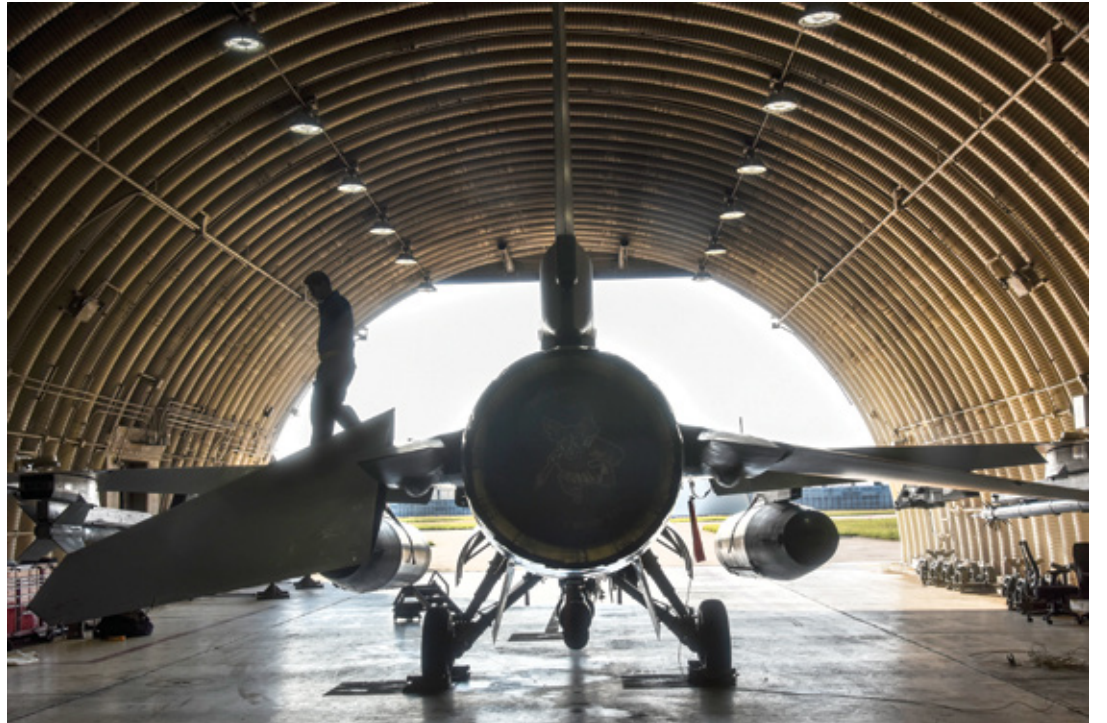
Airman 1st Class Tyler Miller, 80th Aircraft Maintenance Unit crew chief, inspects the wings of an F-16 Fighting Falcon on Kunsan Air Base, Republic of Korea, Sept. 20, 2020. The exterior and interior of the aircraft are examined to ensure that everything is operating properly before and after flying missions. (U.S. Air Force photo by Staff Sgt. Kristin S. High) ▲
