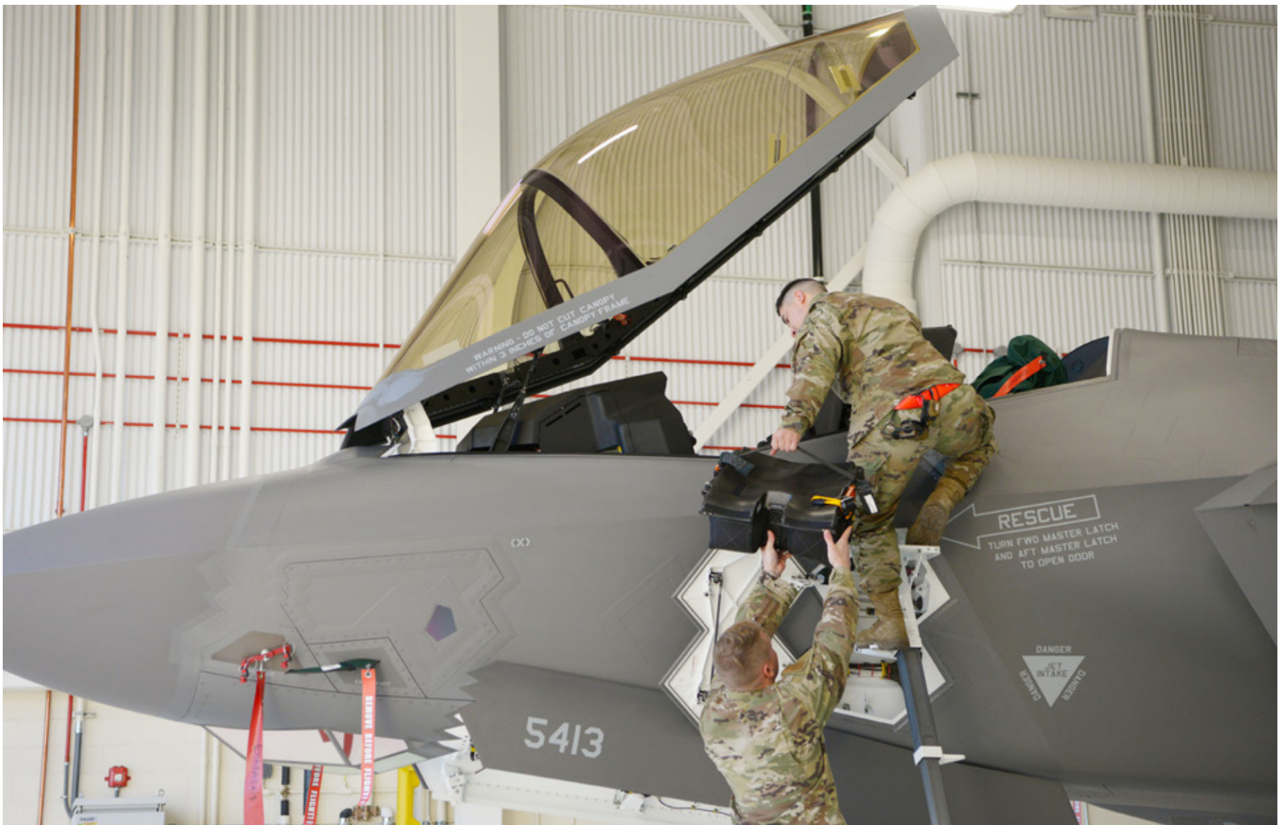
U.S. Air Force Staff Sgt. Victor Benitez, a 354th Maintenance Squadron (MXS) Aircrew Egress journeyman, and Tech. Sgt. Rylee James, a 354th MXS Aircrew Egress F-35A Lightning II cadre member, install the new arctic survival seat kit for the F-35A on Eielson Air Force Base, Alaska, Sept. 28, 2020. Airmen from the 354th Fighter Wing developed a new arctic survival kit for F-35A pilots which is being installed into Eielson’s fleet. (U.S. Air Force photo by Senior Airman Beaux Hebert) ▼
