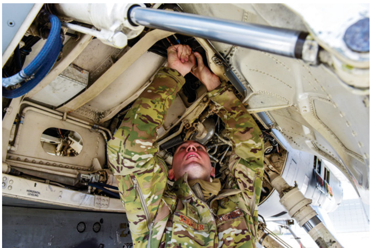
Senior Airman Jacob Scheffler, 80th Aircraft Maintenance Unit electrical and environmental systems journeyman, tightens a bolt to conduct a bleed air ops check on an F-16 Fighting Falcon at Kunsan Air Base, Republic of Korea, Nov. 6, 2020. A bleed air ops check tests air pressure at different points on the jet to verify that the engine swaps over from high-stage to low-stage pressure, and to make sure proper airflow is getting to the cockpit and avionics equipment. (U.S. Air Force Photo by Senior Airman Jessica Blair)
