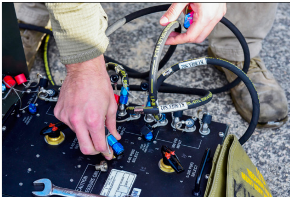
An 80th Aircraft Maintenance Unit electrical and environmental, or E&E, Airman attaches hoses to an environmental control test box at Kunsan Air Base, Republic of Korea, Nov. 6, 2020. E&E personnel attach hoses from the box to the aircraft to run tests on the air pressure. (U.S. Air Force Photo by Senior Airman Jessica Blair) ▲
