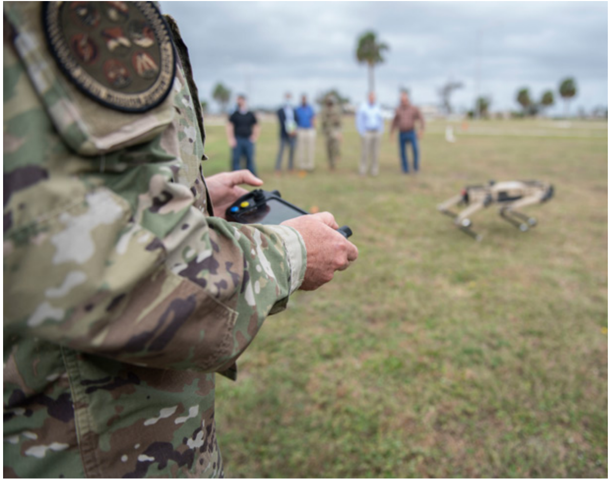
Col. Gregory Beaulieu, 325th Mission Support Group commander, drives an unmanned ground vehicle on Tyndall Air Force Base, Fla., Nov. 10, 2020. Once the robotic UGV are programmed with a path to follow, they will patrol semi-autonomously, only controlled when needed by a virtual-reality headset. (U.S. Air Force photo by Airman 1st Class Tiffany Price)
