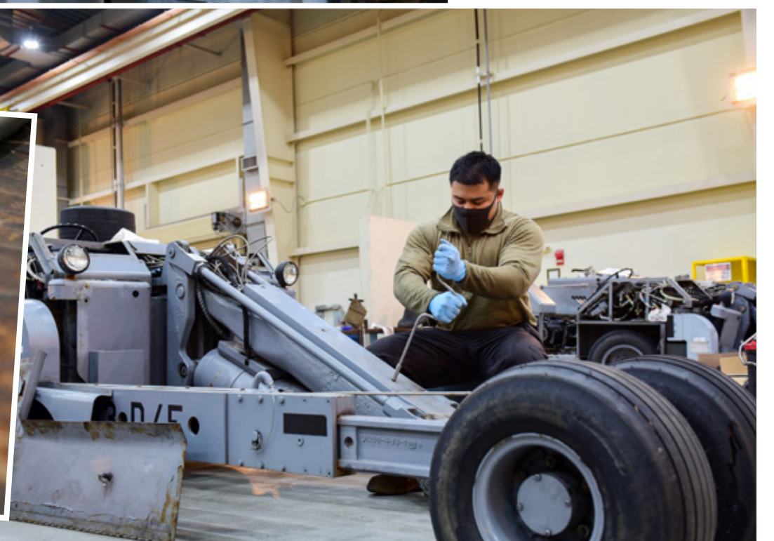
Senior Airman Shane Abalos Villegas, 8th Maintenance Squadron aerospace ground equipment journeyman, removes bolts from a panel on a bombliift vehicle on the flightline at Kunsan Air Base, Republic of Korea, Jan. 21, 2021. Bombliift vehicles are used to transport F-16 Fighting Falcon munitions. (U.S. Air Force photo by Senior Airman Jessica Blair) ▼
