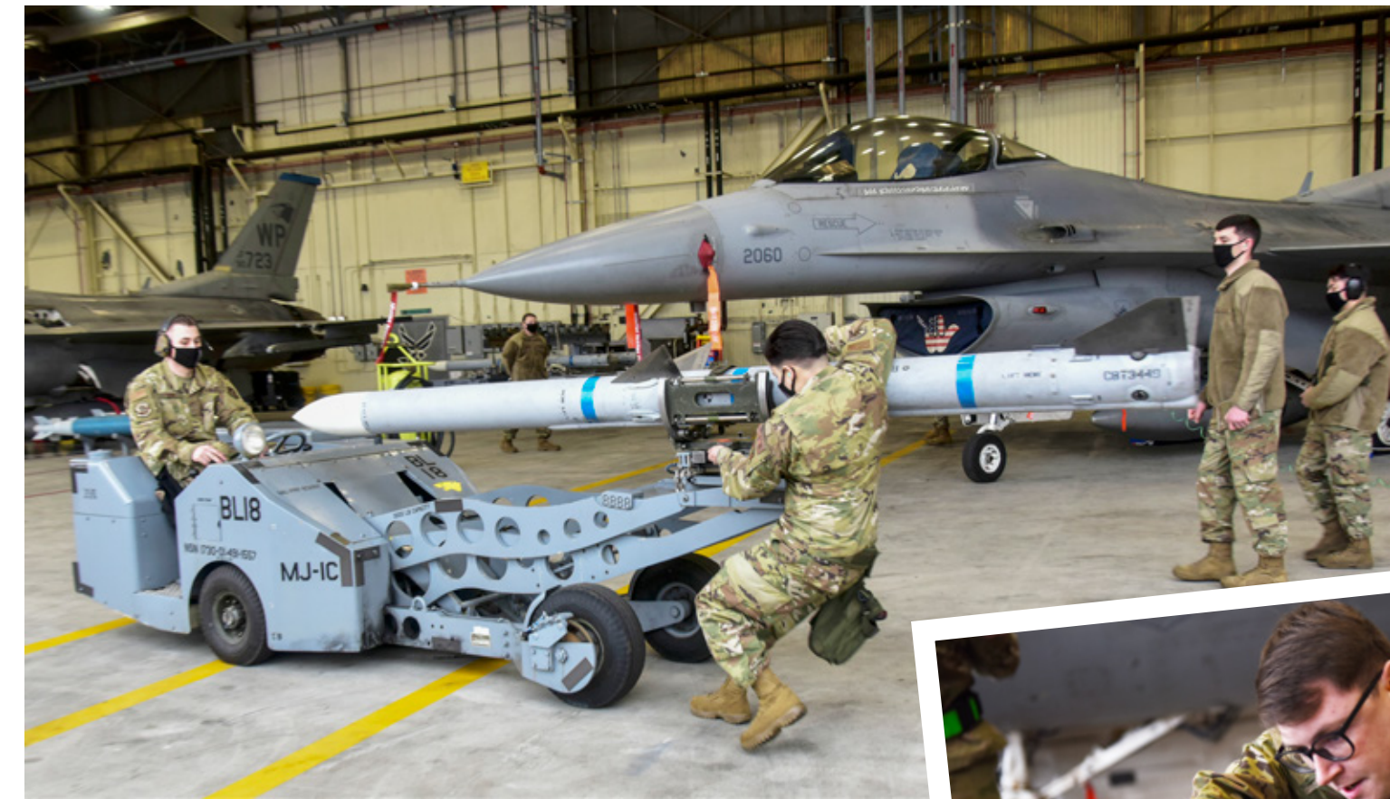
Airmen from the 35th Aircraft Maintenance Unit weapons load crew, transport an AIM 9 L/M Sidewinder with an MJ-1 bomb lift truck during the Annual Load Crew Competition at Kunsan Air Base, Republic of Korea, Feb. 6, 2021. Weapons load crews from the 35th Aircraft Maintenance Unit, 80th AMU and 8th Maintenance Squadron were evaluated on how quickly and effectively they could load munitions onto F-16 Fighting Falcons. (U.S. Air Force photo by Tech. Sgt. Kristin High) ◀
