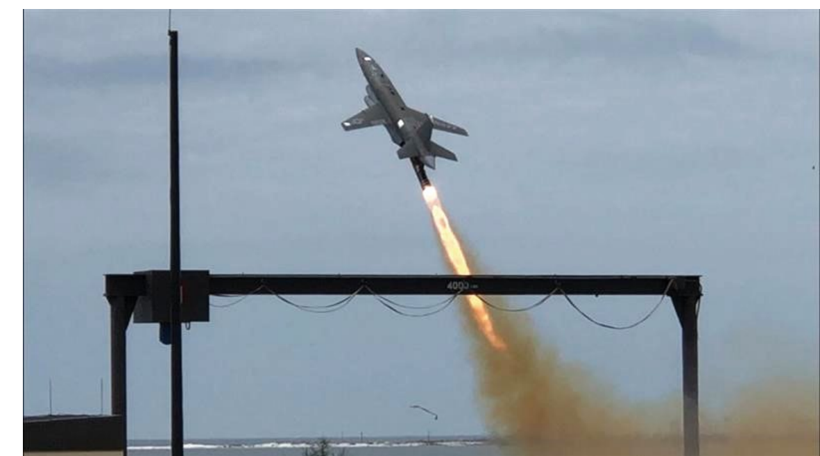
The Skyborg autonomy core system launches aboard a Kratos UTAP-22 tactical unmanned vehicle at Tyndall Air Force Base, Fla., April 29, 2021. The ACS demonstrated basic aviation capabilities and responded to navigational commands, while reacting to geo-fences, adhering to aircraft flight envelopes, and demonstrating coordinated maneuvering. (U.S. Air Force photo) ▲
