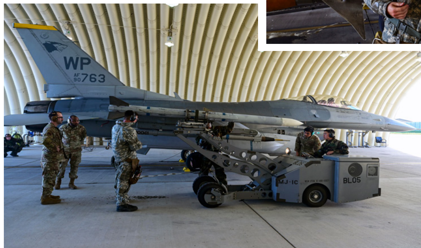
U.S. Air Force Staff Sgt. Jaime Tejada (right), 35th Fighter Generation Squadron weapons load crew team chief, and Airman 1st Class Dimitriy Salomatov, 35th FGS weapons load crew team member, remove a munition from an F-16 Fighting Falcon aircraft at Kunsan Air Base, Republic of Korea, Aug. 7, 2025. During Beverly Sentinel 25-3, Airmen executed integrated combat turns, rapidly loading munitions and refueling the aircraft with engines running to minimize ground time. (U.S. Air Force photo by Senior Airman Karissa Dick) ▲
