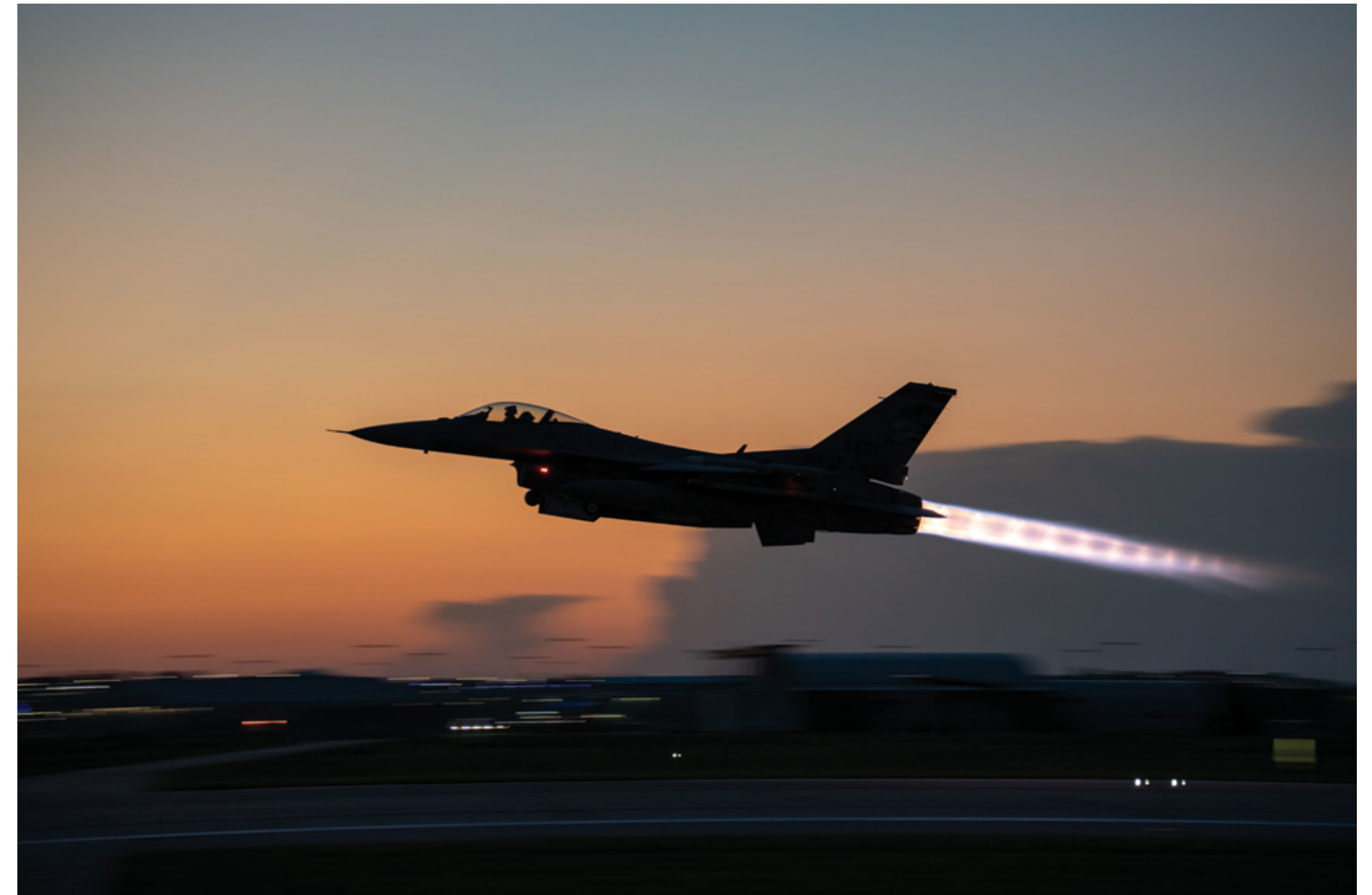
Night flight: An F-16 Fighting Falcon from the 114th Fighter Wing launches into night flying operations with the afterburner engaged at Joe Foss Field, S.D., Aug. 21, 2025. The afterburner provides a significant thrust boost by injecting fuel directly into the exhaust stream, enabling rapid acceleration and high-speed performance essential for combat operations. (U.S. Air National Guard photo by Master Sgt. Luke Olson) ▲
