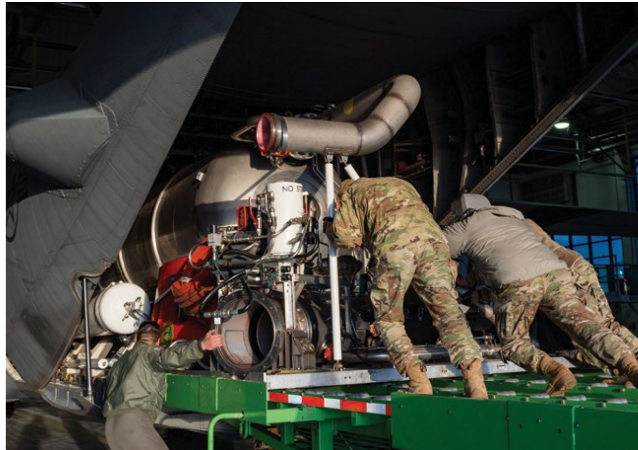
U.S. Air Force Airmen assigned to the 153rd Airlift Wing load and install the Modular Airborne Fire Fighting Systems on to a C-130H Hercules aircraft in Cheyenne, Wyoming, Jan. 10, 2025, in preparation to support firefighting efforts in the Los Angeles area. U.S. Northern Command activated three Wyoming Air National Guard C-130s equipped with MAFFS and associated personnel to assist firefighting efforts in California. MAFFS, developed by the U.S. Forest Service, are portable fire-retardant delivery systems that convert C-130s into airtankers, capable of releasing up to 3,000 gallons of retardant in under five seconds. (U.S. Air Force National Guard photo by Staff Sgt. Zachary Herold) ▲
