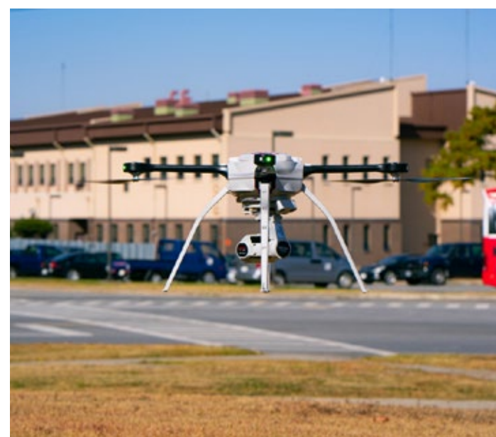
The 51st Civil Engineering Squadron launches a drone to perform a roof inspection outside of Osan Air Base's Turumi Lodge, Nov. 2, 2020. Specialized drones equipped with various camera sensors are being utilized to perform roof inspections across the installation to reduce work hours, remove safety hazards, and simplify the annual process. (U.S. Air Force photo by 1st Lt. Daniel de La Fé) ▲
