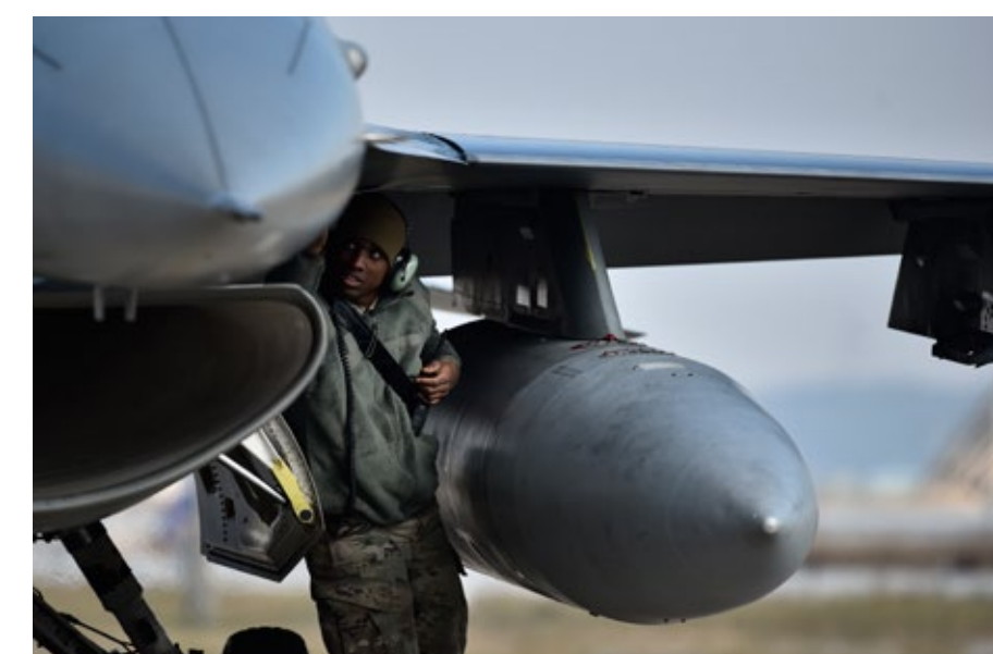
Staff Sgt. Nigel Calhoun, 8th Maintenance Group weapons load crew chief, performs a pre-flight inspection on an F-16 Fighting Falcon at Kunsan Air Base, Republic of Korea, Dec. 10, 2020. Pre-flight inspections are the final step in preparation for an aircraft to take flight. (U.S. Air Force photo by Senior Airman Mya M. Crosby) ▲
