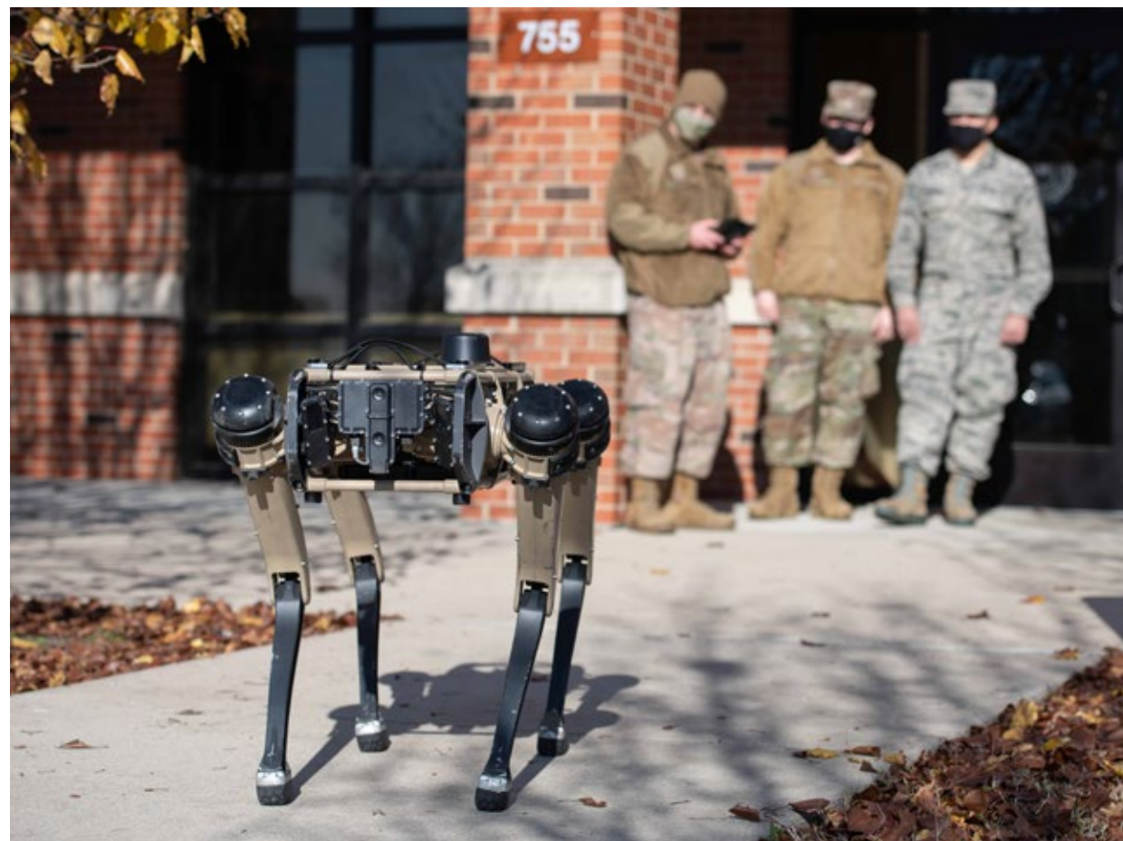
Airmen assigned to the 375th Security Forces Squadron function check the Ghost Robotics Vision 60 semi-autonomous robot dog before a demonstration at Scott Air Force Base, Ill., Dec 14, 2020. The robot dog utilizes an adaptive communication system allowing the machine to operate on a series of preset commands or when operated manually. (U.S. Air Force photo by Airman 1st Class Shannon Moorehead)
