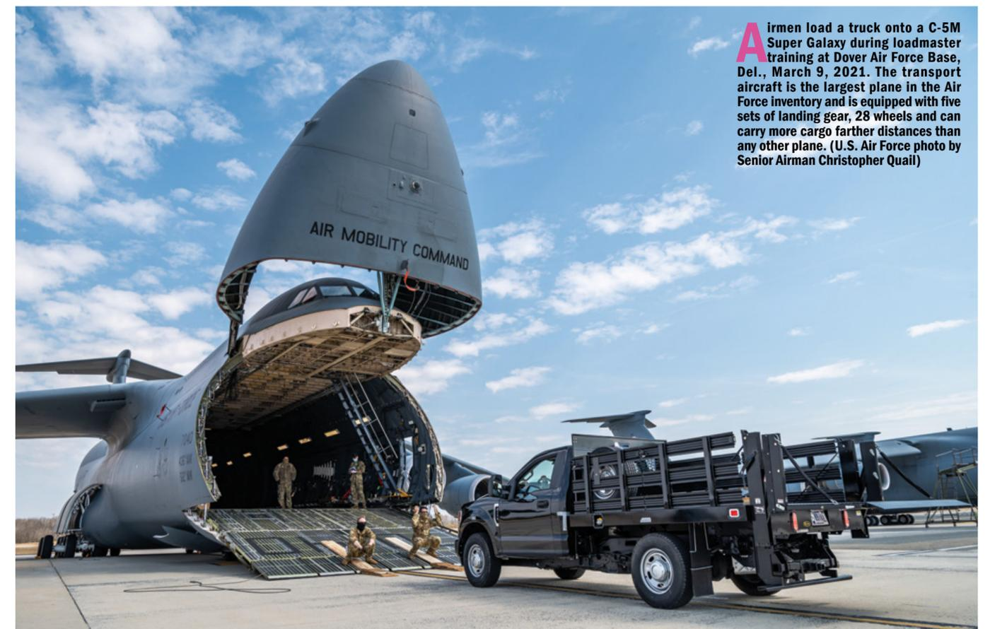
**A**irmen load a truck onto a C-5M Super Galaxy during loadmaster training at Dover Air Force Base, Del., March 9, 2021. The transport aircraft is the largest plane in the Air Force inventory and is equipped with five sets of landing gear, 28 wheels and can carry more cargo farther distances than any other plane. (U.S. Air Force photo by Senior Airman Christopher Quail)
