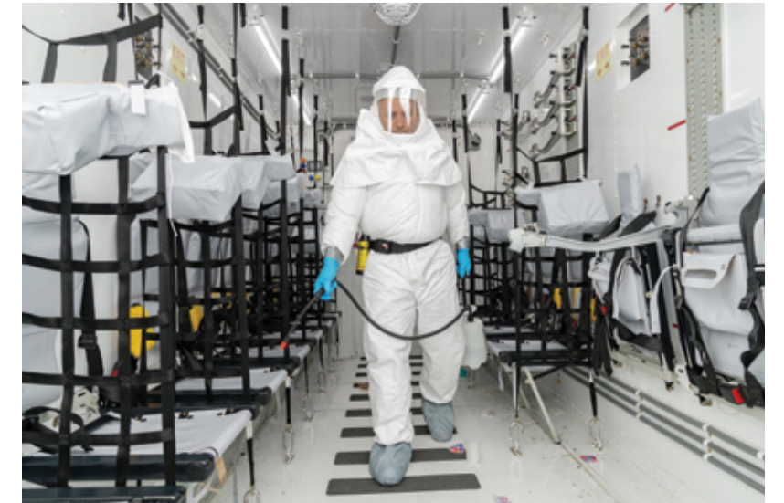
Master Sgt. Leonardo Erazo, 5th Health Care Operations Squadron medical logistics flight chief, simulates decontaminating the inside of a Negatively Pressurized Conex loaded on a C-17 Globemaster III at Dover Air Force Base, Del., April 7, 2021. NPC's are containment units designed to allow in-flight medical care for patients with diseases like COVID-19 while minimizing the possible spread of infectious diseases to medical personnel and aircrew on board. (U.S. Air Force photo by Roland Balik)
