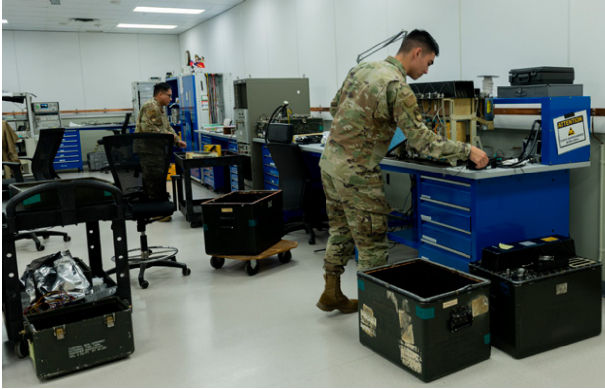
U.S. Air Force Senior Airman Bryant De Los Reyes, 51st Maintenance Squadron precision measurement equipment laboratory logistics technician, changes out a circuit in a joint service electronic combat systems tester at Osan Air Base, Republic of Korea, Dec. 15, 2023. The PMEL flight calibrates nearly every piece of equipment in every phase of maintenance. (U.S. Air Force photo by Senior Airman Kaitlin Castillo) ▲
