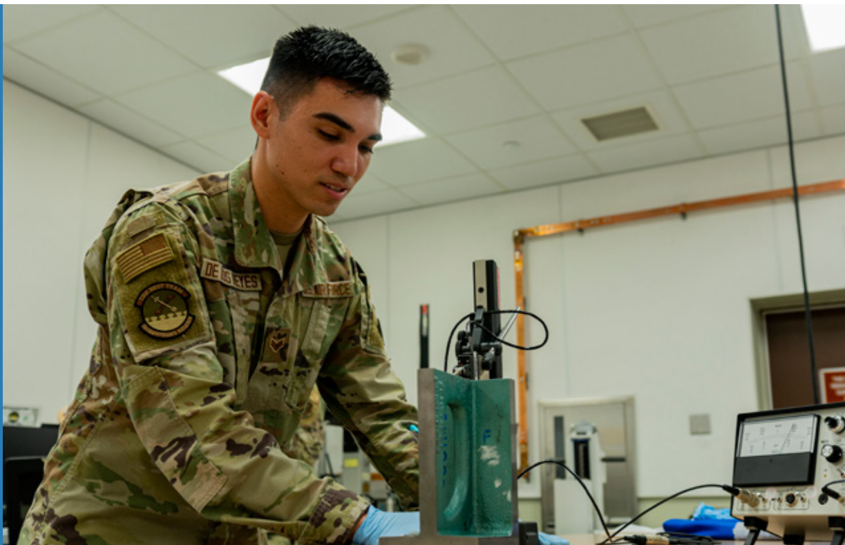
U.S. Air Force Senior Airman Bryant De Los Reyes, 51st Maintenance Squadron precision measurement equipment laboratory logistics technician, compares the parallelism of an angle iron at Osan Air Base, Republic of Korea, Dec. 15, 2023. The PMEL flight services more than 100 organizations at Osan and across the ROK. (U.S. Air Force photo by Senior Airman Kaitlin Castillo) ▲
