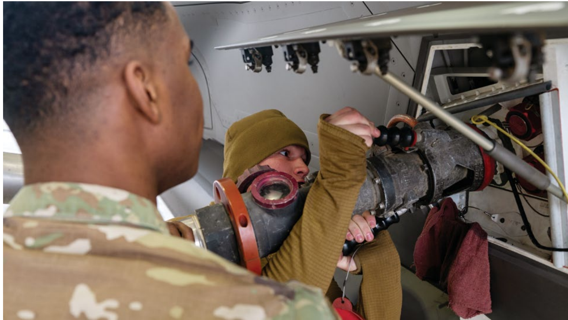
U.S. Marine Lance Cpl. Nathan Jones, right, Marine Wing Support Squadron 172 motor transportation operator, and U.S. Air Force Senior Airman Andre Franklin, 8th Logistics Readiness Squadron fuels distribution technician, fasten a fuel hose to an F-35A Lightning II at Kunsan Air Base, Republic of Korea, Feb. 22, 2024. In tandem with the combined training mission U.S. Air Force and ROK Air Force pilots were conducting, Airmen assigned to the 8th LRS provided airfield familiarization and mission integration training to Marines currently embedded into their unit. (U.S. Air Force photo by Staff Sgt. Samuel Earick) ▲
