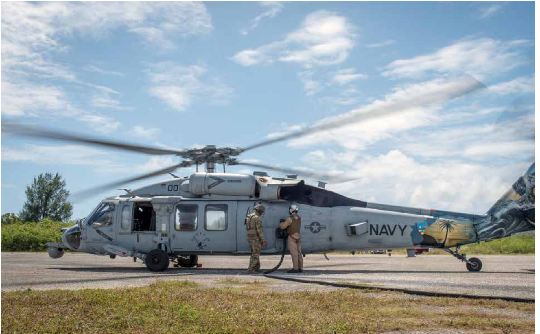
A U.S. Navy MH-60S Seahawk, assigned to the Helicopter Sea Combat Squadron 25, is refueled by a helicopter expedient refuel system (HERS) during exercise COPE NORTH 2018 at Tinian, U.S. Commonwealth of the Northern Mariana Islands, Feb. 26. A HERS is a deployable fueling system capable of storing 3,000 gallons of fuel. (U.S. Air Force photo by Airman 1st Class Juan Torres Chardon)
