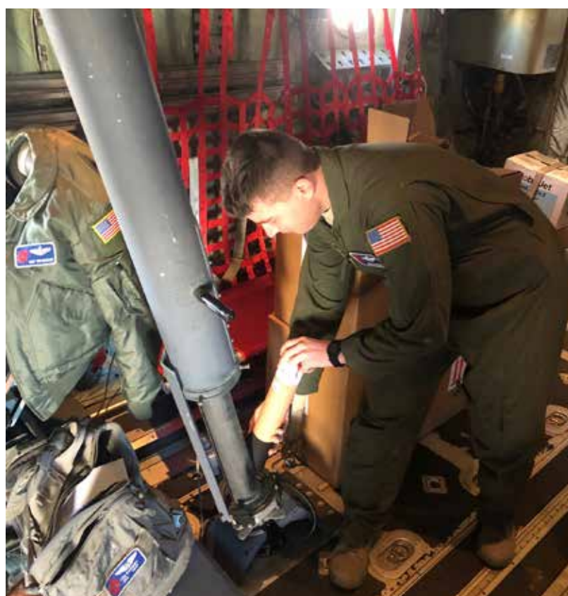
Master Sgt. Thomas Barnaby, 53rd Weather Reconnaissance Squadron loadmaster, loads a dropsonde into a dropsonde cannon aboard a WC-130J Super Hercules Aircraft Jan. 26, 2018 above the Pacific Ocean during an atmospheric river mission. (U.S. Air Force courtesy photo)
