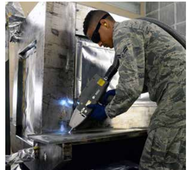
Airman 1st Class Levi Gordon, 60th Maintenance Squadron aircraft structural maintenance, uses a Clean Laser 1000 to remove paint from a sheet of metal March 7, 2018, at Travis Air Force Base, Calif. The 1000-watt laser can remove paint and corrosion and reduces the waste created from sanding paint by 90 percent. Travis AFB was chosen as one of two bases to test the capabilities of the laser. (U.S. Air Force photo by Staff Sgt. Amber Carter)
