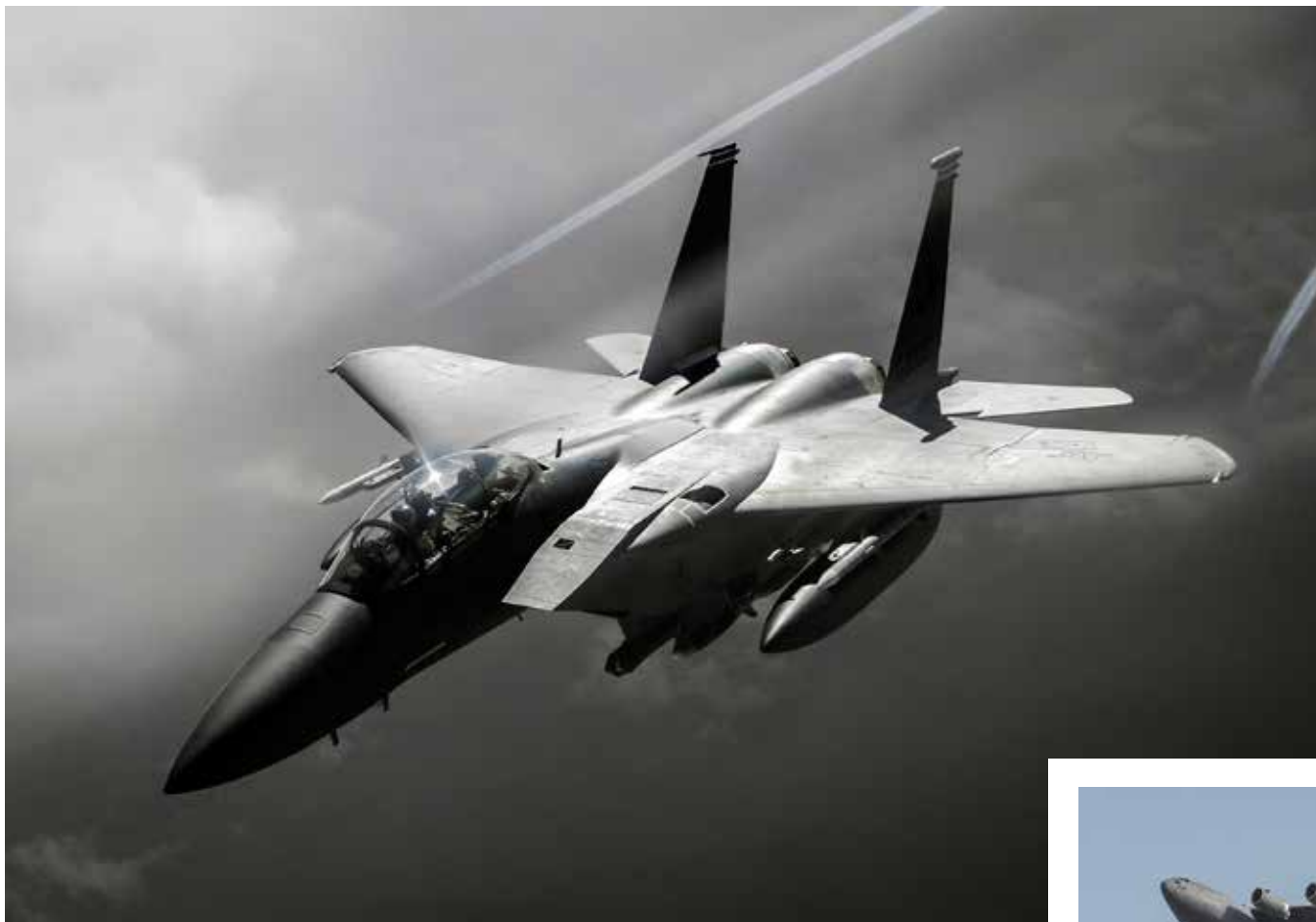
A U.S. Air Force F-15E Strike Eagle flies over Iraq on May 5, 2018. The F-15E is a dual-role fighter designed to perform air-to-air and air-to-ground missions. An array of avionics and electronics systems gives the F-15E the capability to fight at low altitude, day or night, and in all weather. (U.S. Air Force photo by Staff Sgt. Corey Hook) ◀
